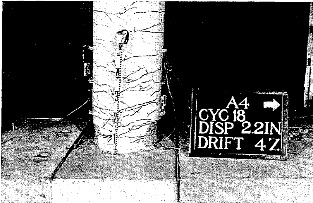
FIGURE 4-13 Condition of Specimen A4 at Cycle No. 18
