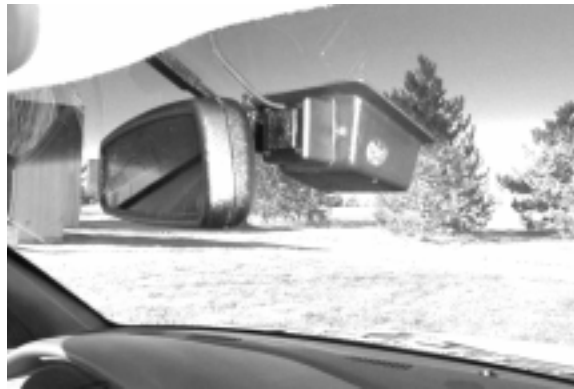
Figure 20. Forward-looking CCD camera
