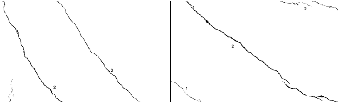
Figure 9.5 Final Crack Image of TNRPi1 at 319 kips (S3 & S2)
