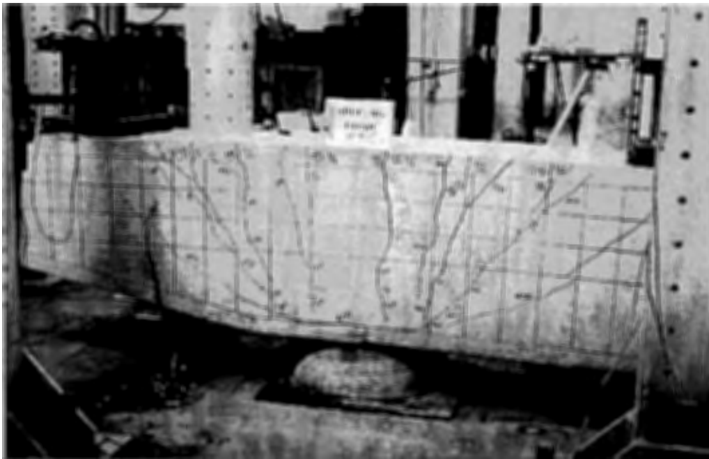
Figure E-27. Specimen 8G Cracking Pattern at P = 440 kips.
