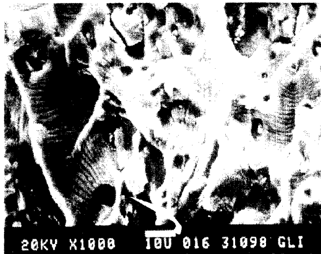
SEM photo of corrosion fatigue of aluminum alloy
