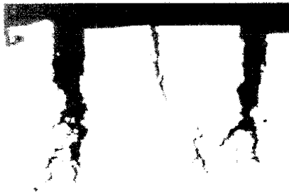
Transgranular stress-corrosion cracking
