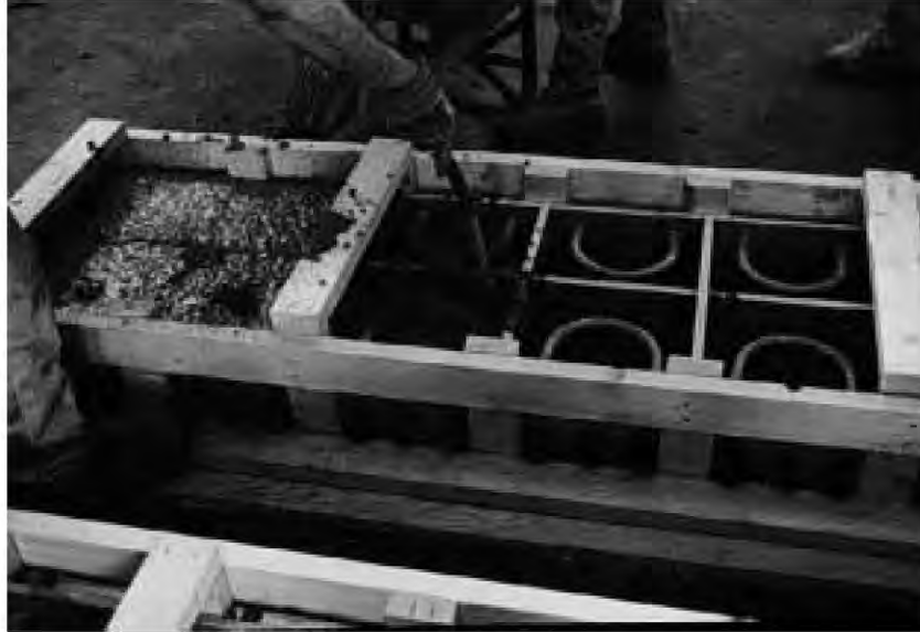
Figure A.15 Casting macrocell specimens.
