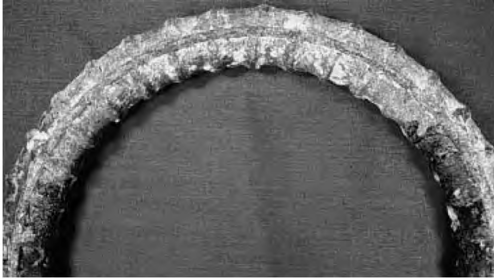
(a) Uncoated bar free of rust at bend
