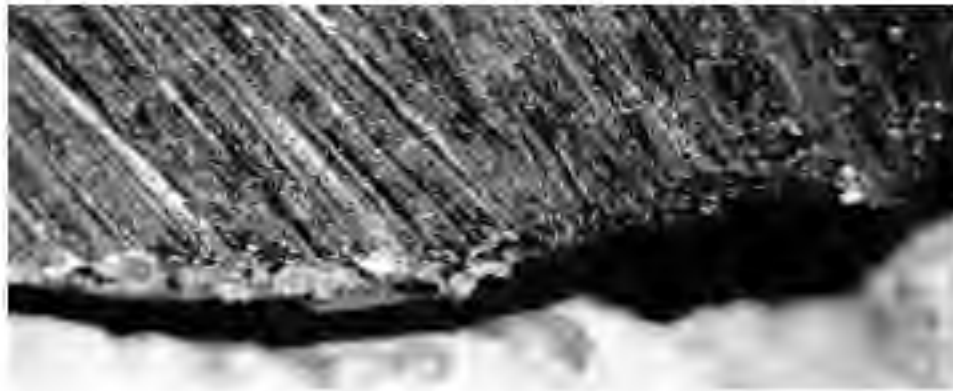
Figure 3.26 Gap formation below coated bar.
