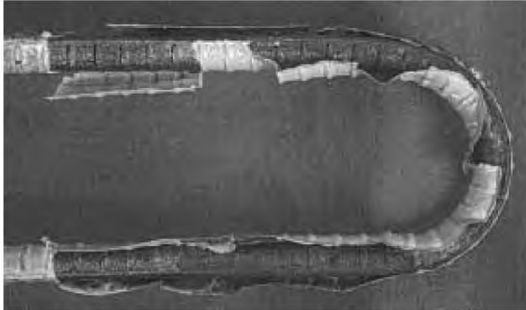
Figure 2.34 Coating debonding on 13-mm (#4) bar.
