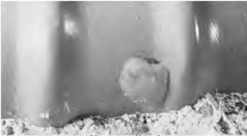
(a) Blister on a coated bar surface
