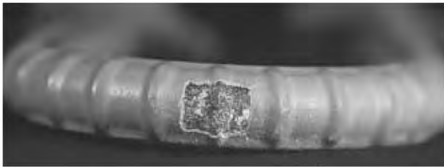
Figure 2.25 Clean, uncorroded damaged area after 4.5 years of exposure (Bar 3A.3).
