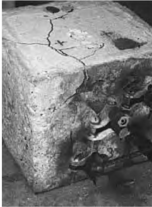
Figure 2.8 Surface condition of specimen with uncoated bar.
