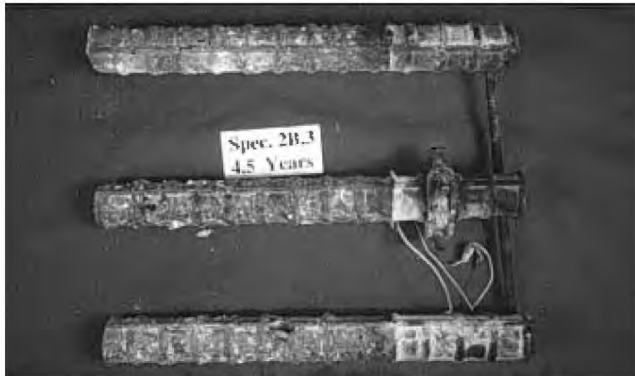
Figure 2.33 Appearance of bottom side of cathodic, bottom bars of specimen 2B.3.
