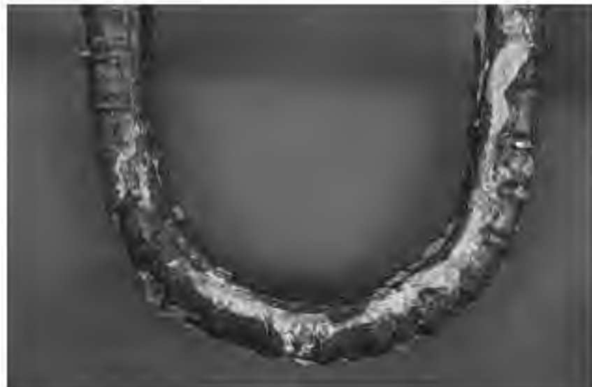
Figure 2.44 Whitish products alongside longitudinal lug at bottom side of bar 1A.5.
