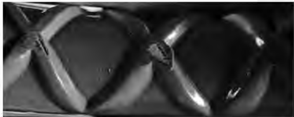
(b) Bar with cross deformations
