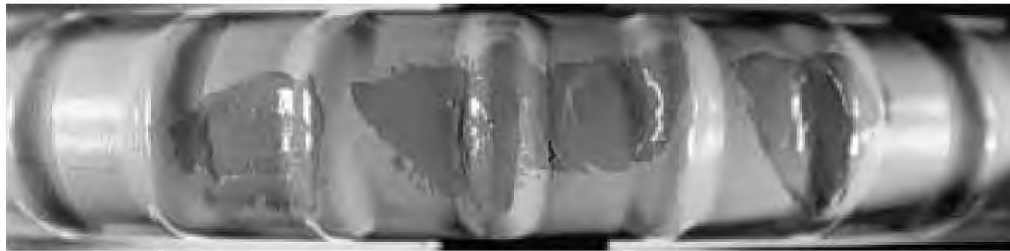
(a) Damage spots > 6x6 mm, bar with parallel deformations
