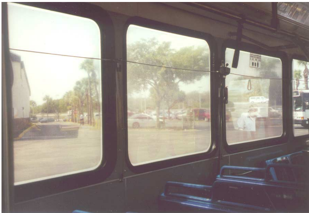
Picture 22 From inside an ad wrapped bus, the outside view appears blurred. The distortion is worse at night for customers trying to see landmarks or read street signs. The interior is darkened due to both tinted glass and full wrap advertising. Would a return to clear glass lead to a more secure environment?
