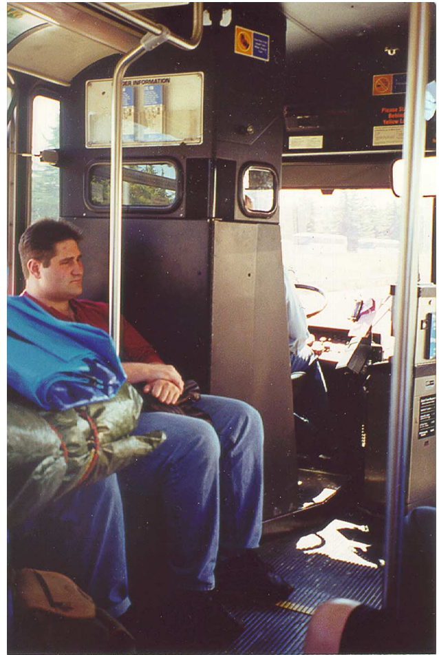
Picture 20 King County Metro's articulated buses supplied by Breda provide a small extension of the modesty panel towards the front. This reduces glare from interior lighting at night, but is not an explicit security feature.
