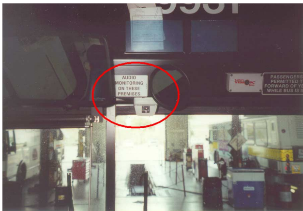
Picture 6 A camera mounted at the front of the bus provides a view of the entire interior.
