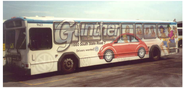
Picture 21 A typical transit bus with full wrap advertising. Note the operator's window is left uncovered.
