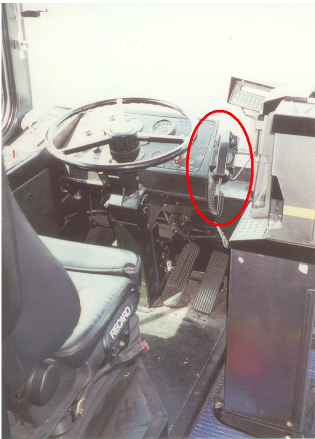
Picture 1 A typical bus operator's workstation includes a 2-way radio for voice communications with dispatch. Note the farebox on the right.
