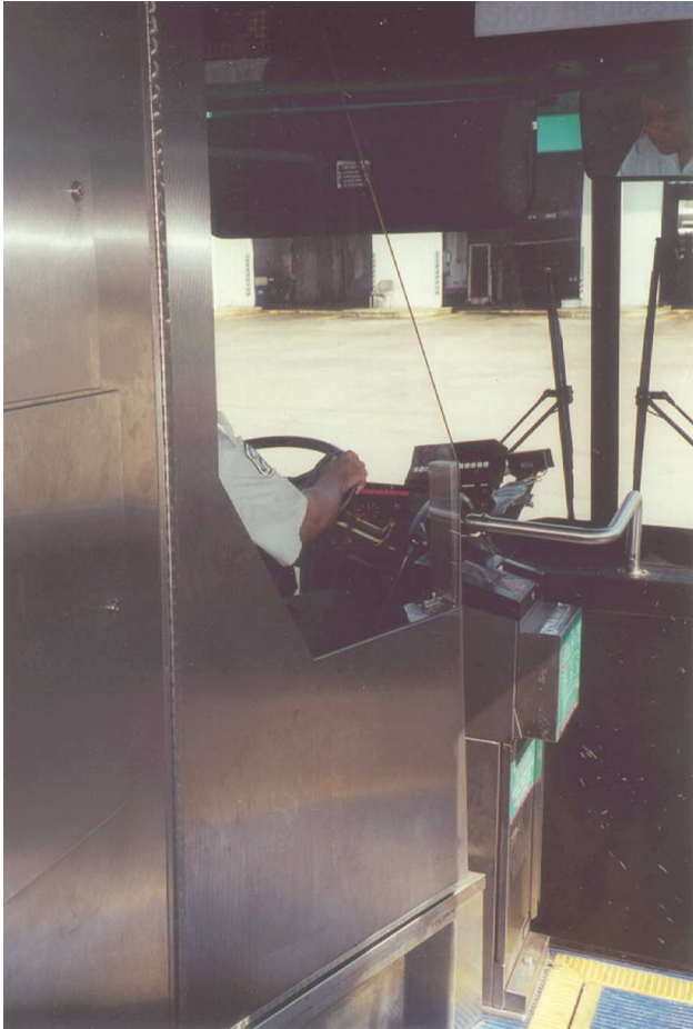
Picture 15 The door and panel is designed to address potential threats from the operator's blind spot.
