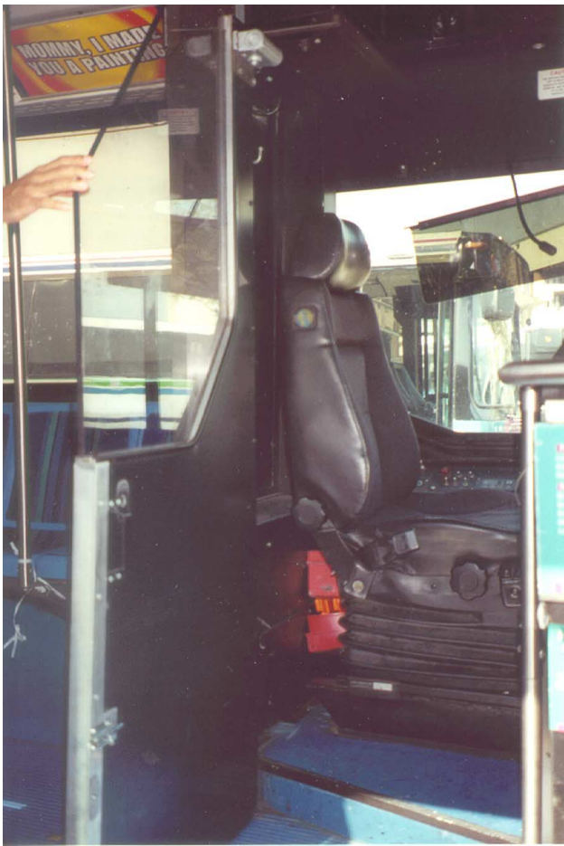
Picture 19 Some MDT operators tie the doors open. The door may also present an obstacle for maintenance cleaning staff.
