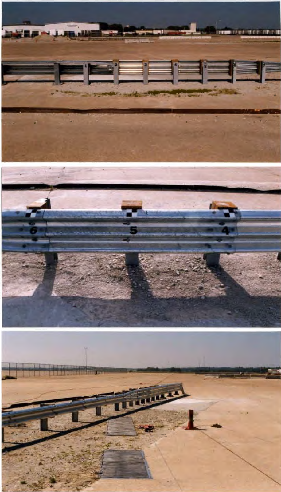
Figure 11. W-beam to Thrie Beam Transition (Continued)
