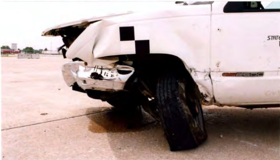
Figure 52. Vehicle Damage, Test MWT-2
