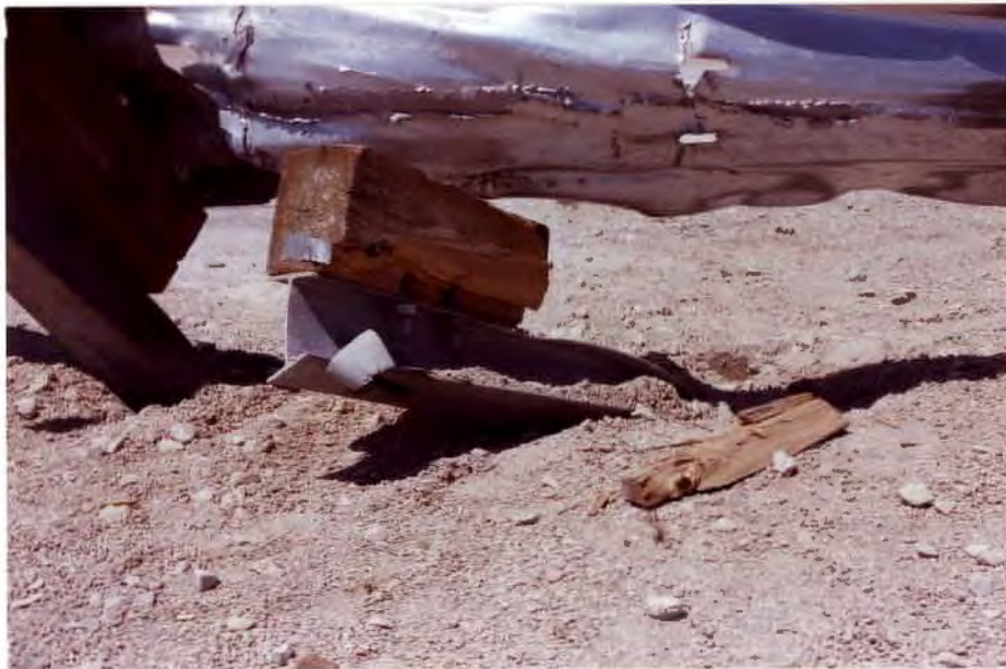
Figure 48. Post No. 6 and 7 Damage, Test MWT-2
