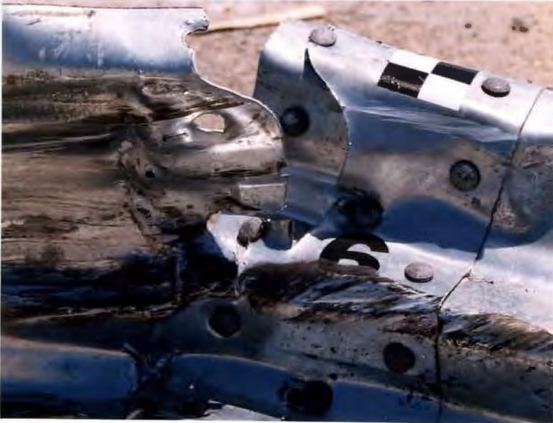
Figure 46. W-beam to Thrie Beam Transition Damage, Test MWT-2
