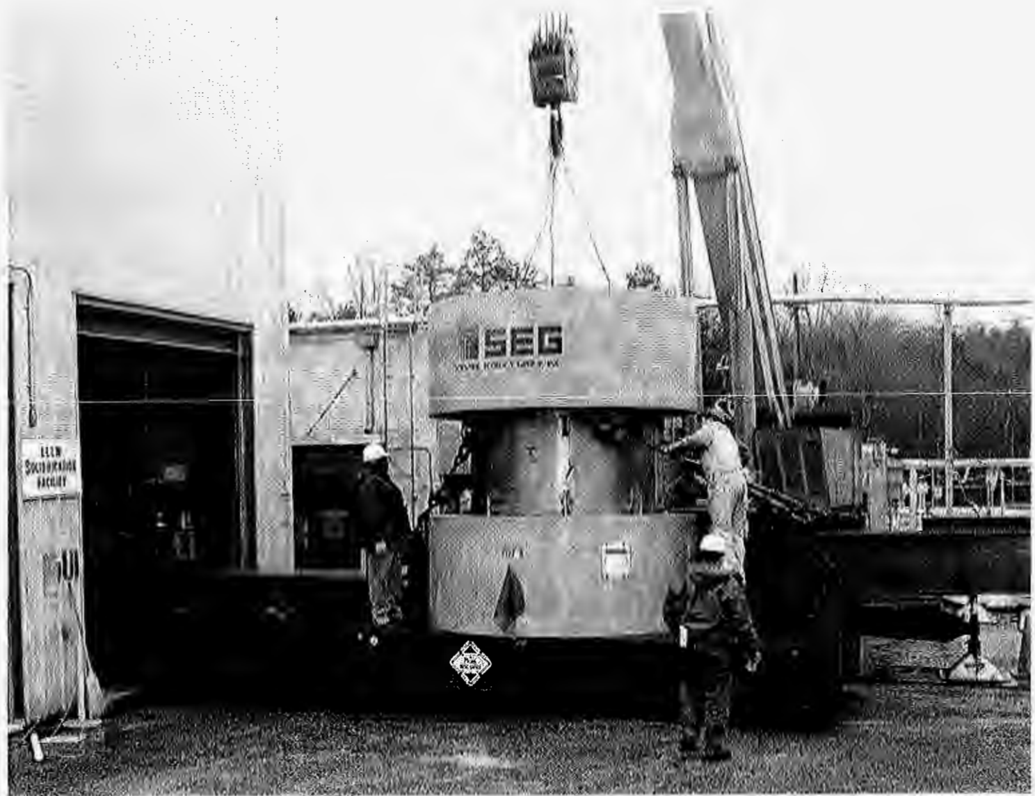
Fig. 18. Photograph of a loaded type B carrier being prepared for shipment to SRS.
