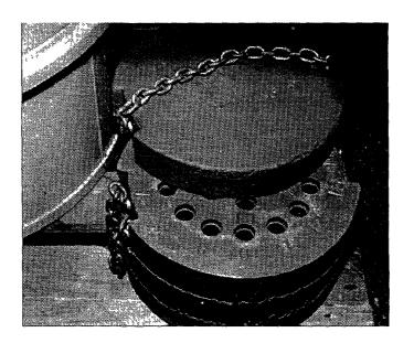
FIG. A-6. Lead shielding device for storage.
