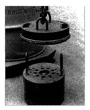
FIG. A-5. Lead shielding device for storage.
