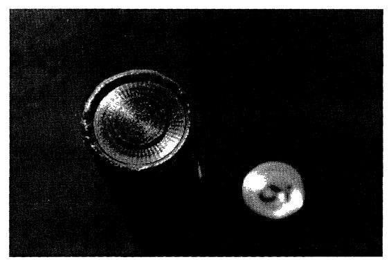
FIG. A-3. Welded stainless steel capsule.
