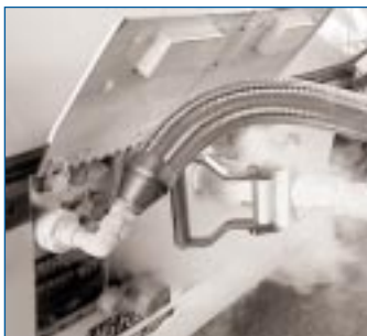
Figure 8. LNG fueling hoses connected to DART bus
