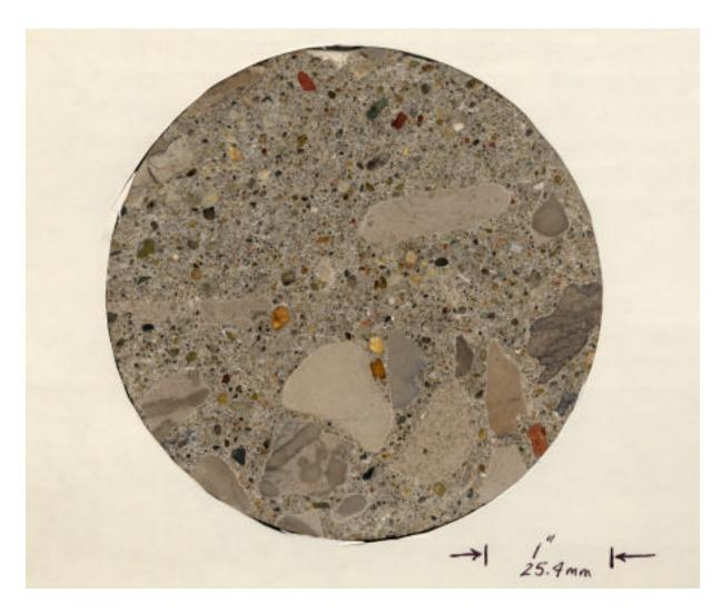
FIGURE 8 Illustration of segregation in a core extracted from I-80 in Iowa county.
