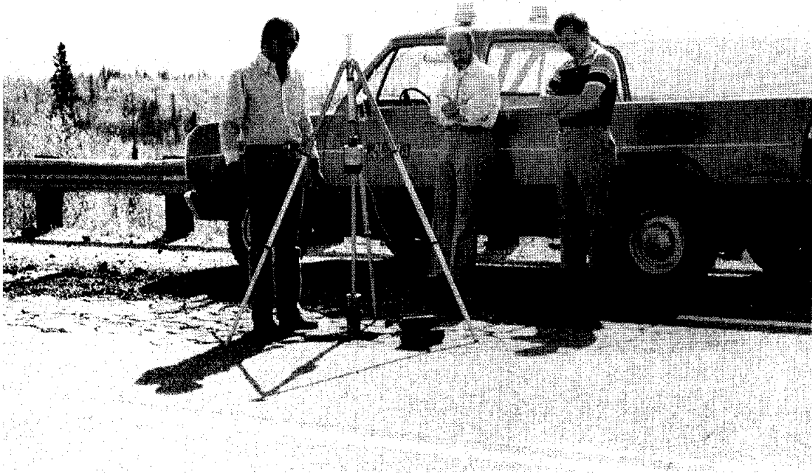
FIGURE 9. Testing Base Course Materials with a Small Falling Weight Deflectometer
