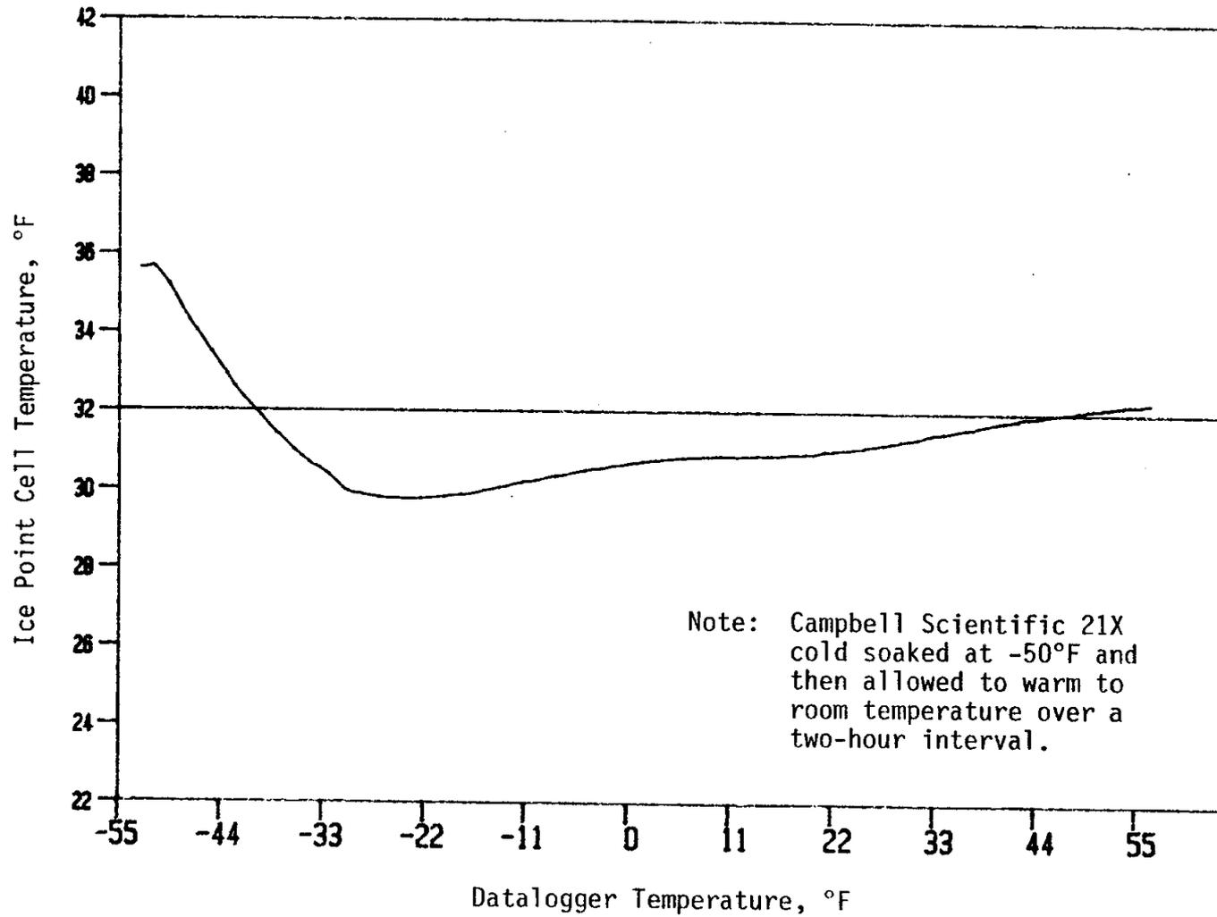
Figure 4. Campbell accuracy as a function of temperature during a warming cycle.
