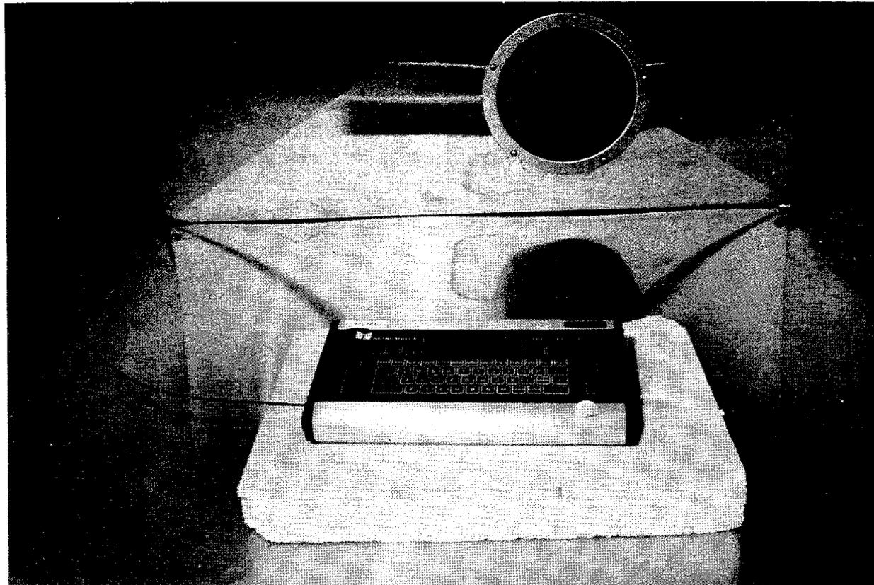
Figure 2. Metrosonics dl-721 datalogger on expanded polystyrene insulation inside environmental test chamber.
