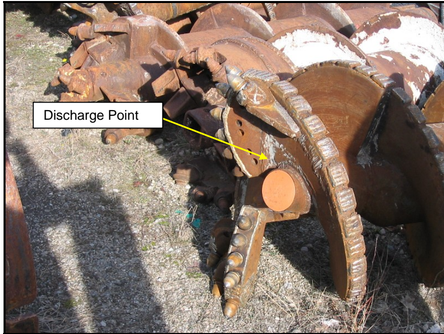
Figure 4.10: Hardened Cutting Head
