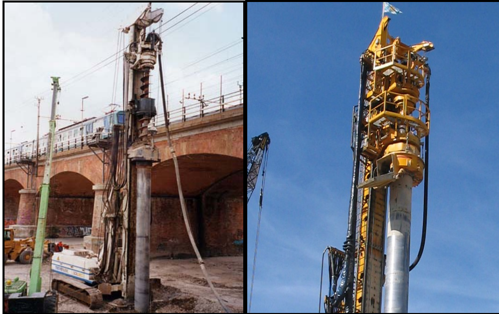
(a) Movable Rotary Drive (b) Fixed Twin Drive
