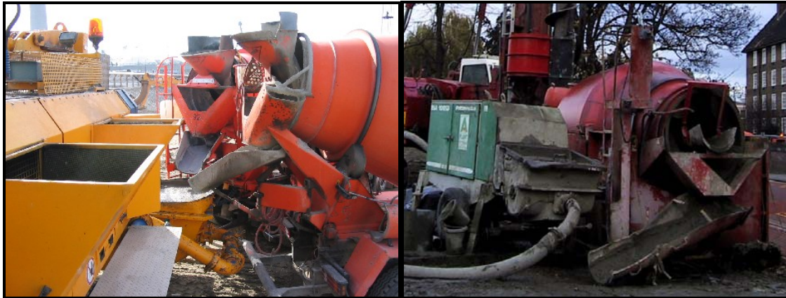
(c) Concrete Pump Mounted on Rig
