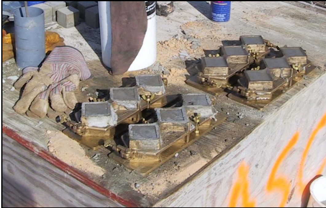
Figure 7.10: Cubes for Grout Testing
