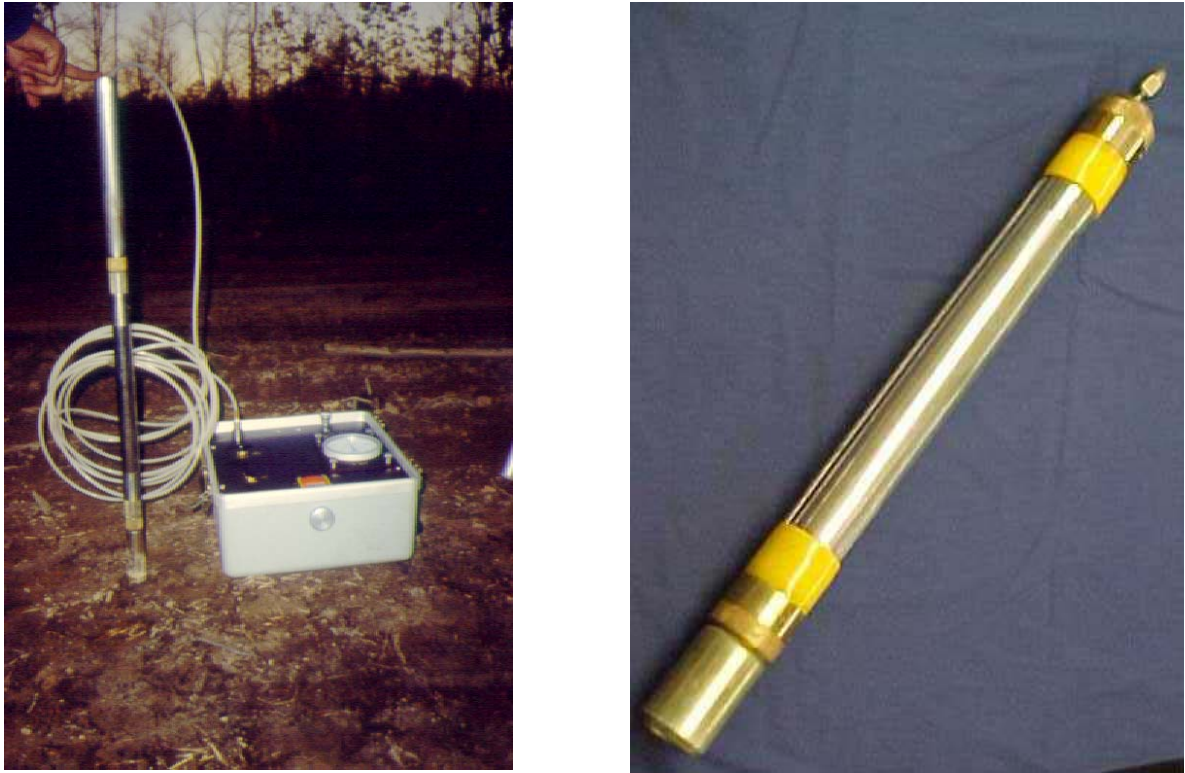
Figure 17. Pre-bored pressuremeter equipment.
