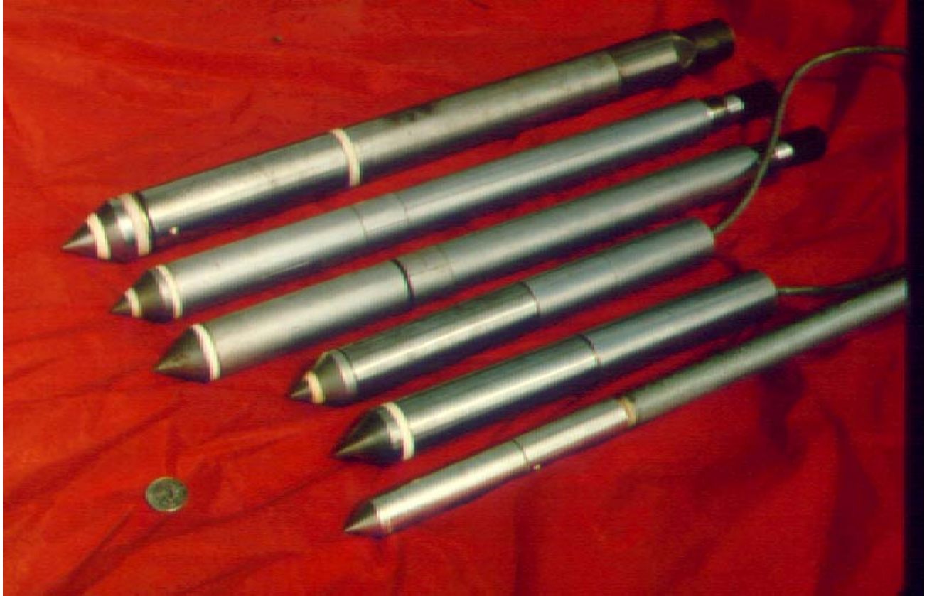
Figure 12. Cone and piezocone penetrometers (note the quarter for scale).
