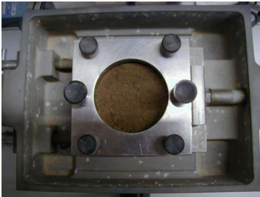
Figure 30. Soil sample mounted in direct shear testing apparatus (photograph courtesy of GeoTesting Express).
