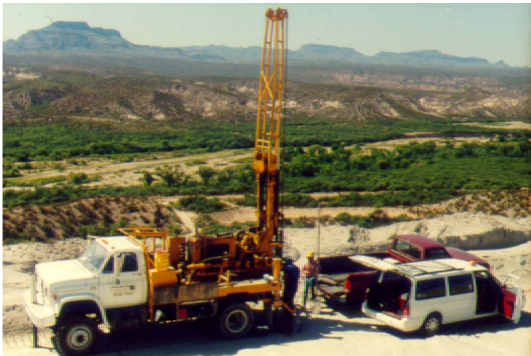
Figure 10. SPT performed at the back of a drill rig.
