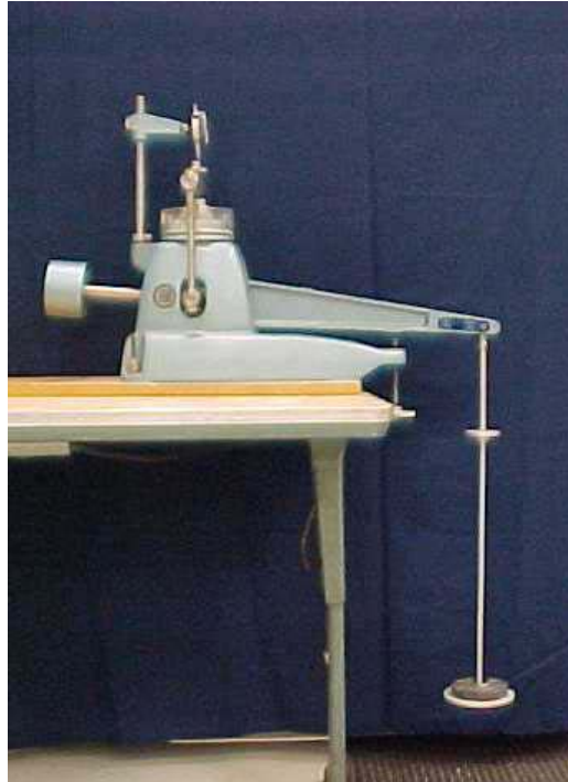
Figure 27. Incremental load oedometer.
