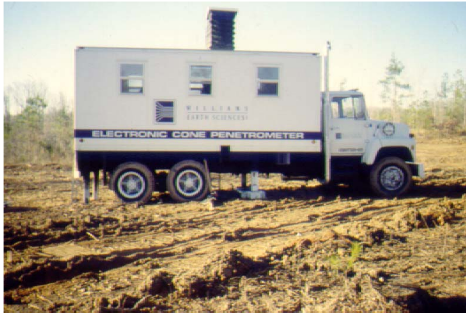
Figure 13. Cone penetration testing from cone truck.
