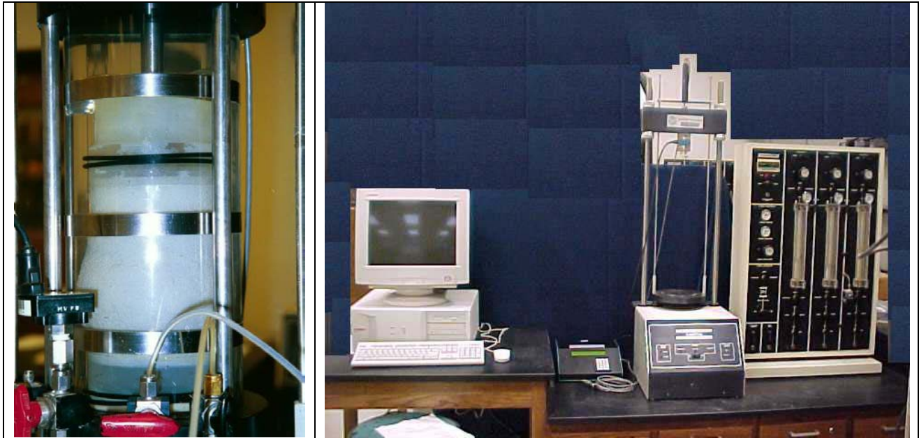
Figure 28. (a) Failure of a loose sand specimen in a triaxial cell; and (b) Load frame, pressure panel, and computerized data acquisition system
