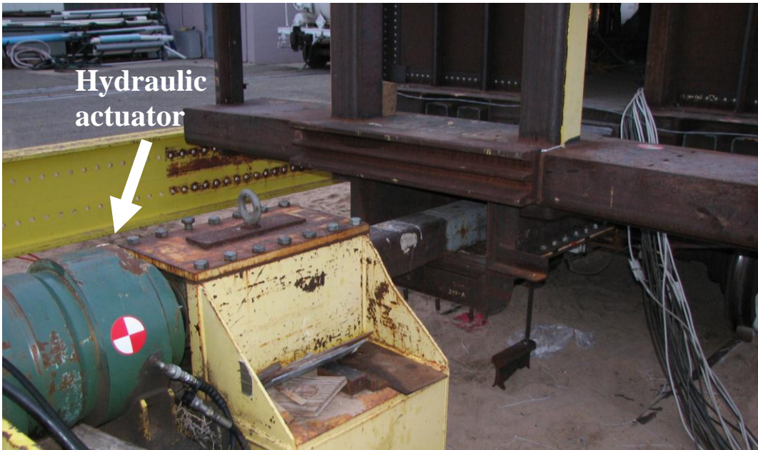
Figure 3. Test Setup at Load Application End
