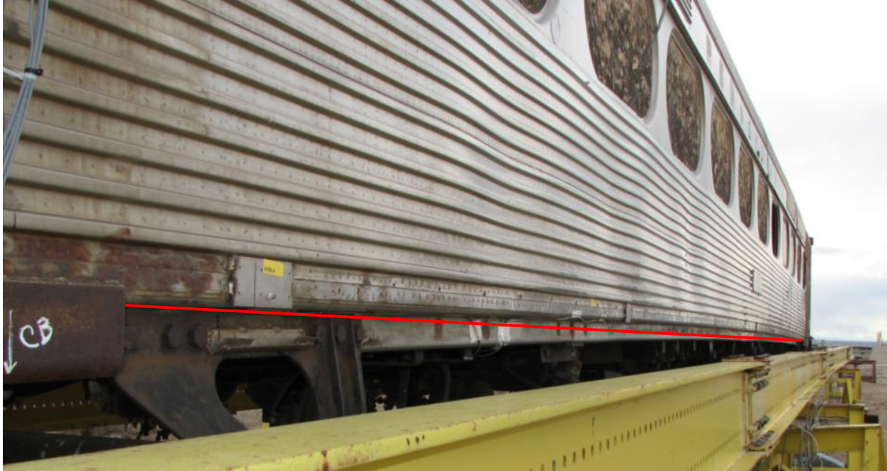
Figure 15. The Test Car under 800,000-Pound Compressive Load
