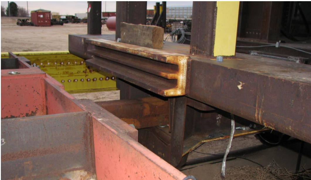
Figure 4. Test Setup at Load Reaction End
