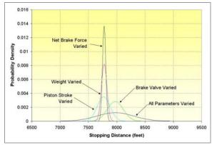
Figure 3. Stopping Distances for a Long, Loaded, General Freight Train Stopping from 60 mph on Flat Grade
