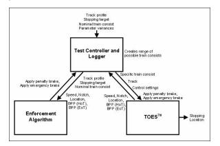
Figure 2. Simulation Test Environment
