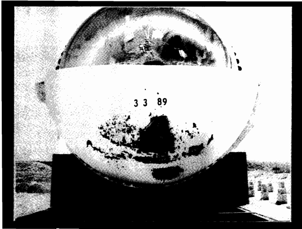
FIGURE 16. 111 SHIELDED HEAD FA-21 PUNCTURE - IMPACT SPEED 17.8 MPH - 1/2"-THICK SHIELD.
