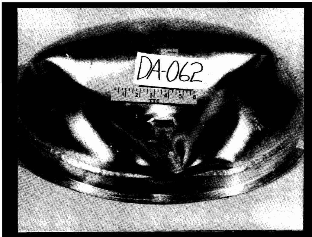
FIGURE 36. VIEW OF PUNCTURED 111 HEAD WITH JACKET REMOVED - NOTE FOLDING AND PINCHING AT SILL AREA.
