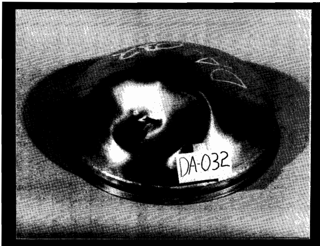
FIGURE 31. TYPICAL PUNCTURE OF 111 BARE ALUMINUM HEAD.
