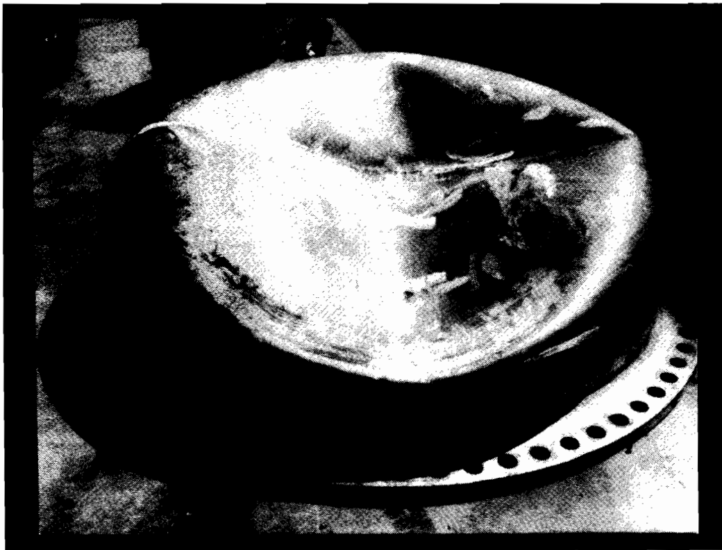
FIGURE 21. FA-31 HEAD, SHIELD REMOVED - NOTE DEFORMATION AT SILL AREA.
