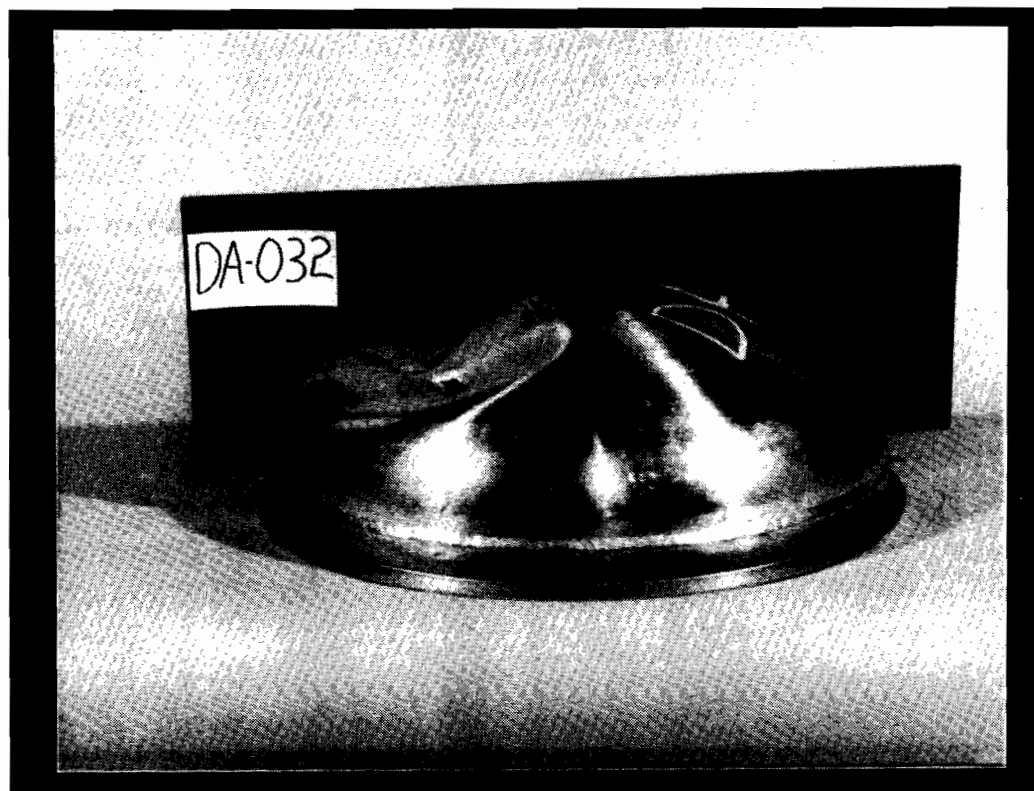
FIGURE 32. PROFILE TEMPLATE USED TO MEASURE DENT DEPTH.
