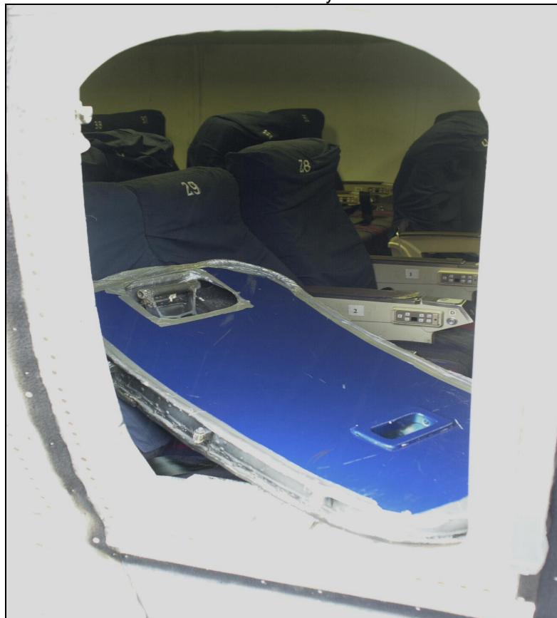
Figure 29 Exit Obstructed by Hatch
