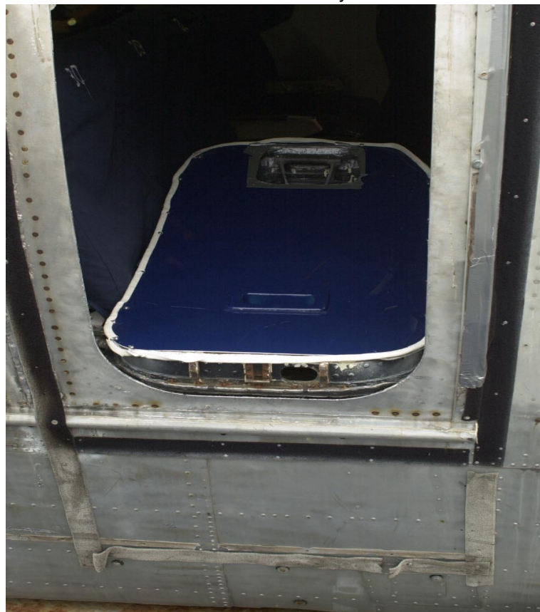
Figure 30 Slide to Exit Formed by Hatch
