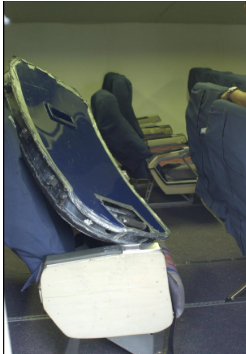
Figure 5 Typical Inside Hatch Disposal Location
