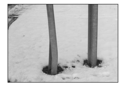
In this case, the slip base supports are under several inches of back fill, consequently failed to activate when hit, note the bending of the left leg.
