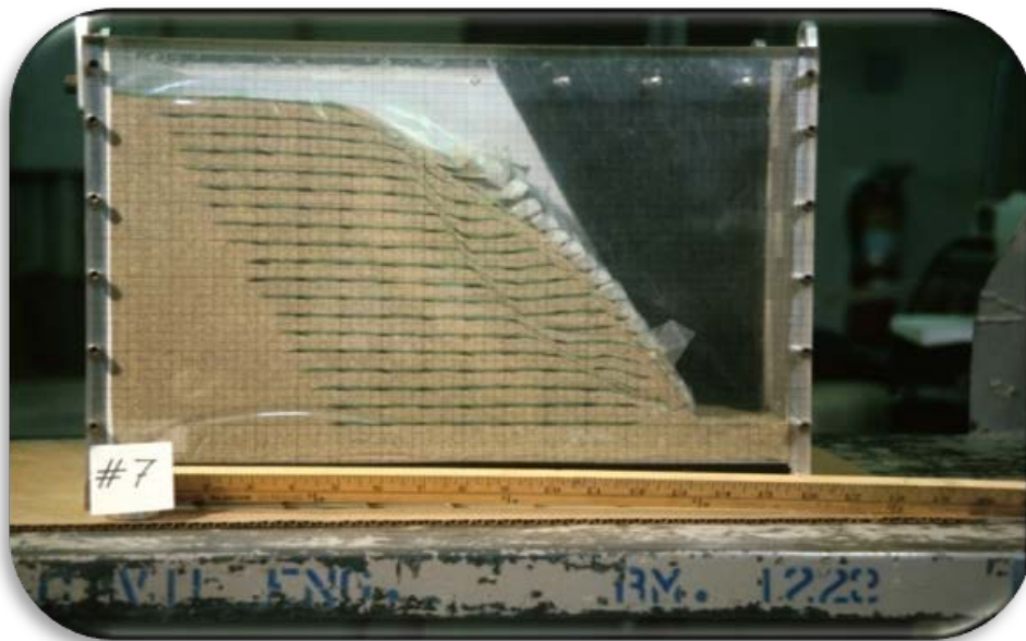
Figure 4-4. Failed geotextile-reinforced slope/wall in centrifuge modeling (courtesy Prof. Zornberg)
