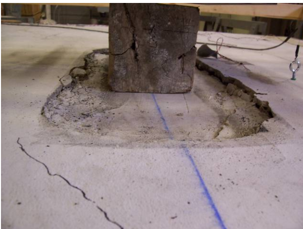
Figure 14 – Imprint of punching shear failure initiation on specimen G1
