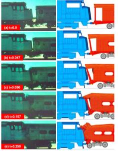
Figure 7. Comparison of Test and Analysis Results
