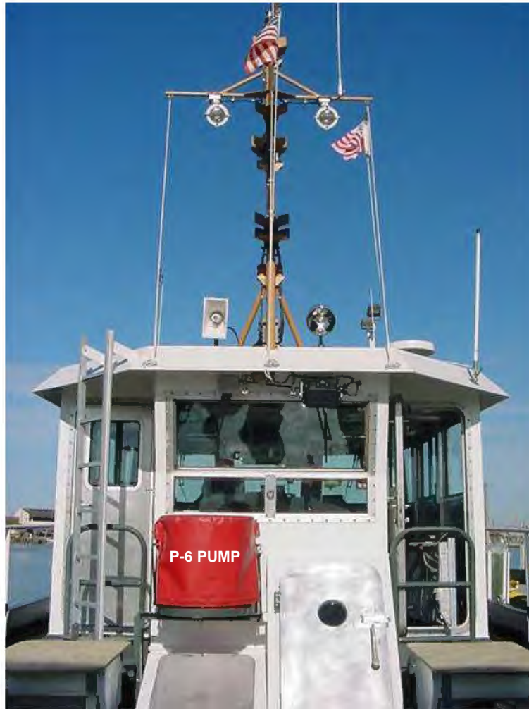
Figure 2-25 Emergency Dewatering Pump
