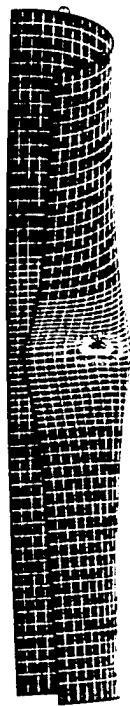
Figure 11: Equivalent plastic strains in the pipe wall after impact.
