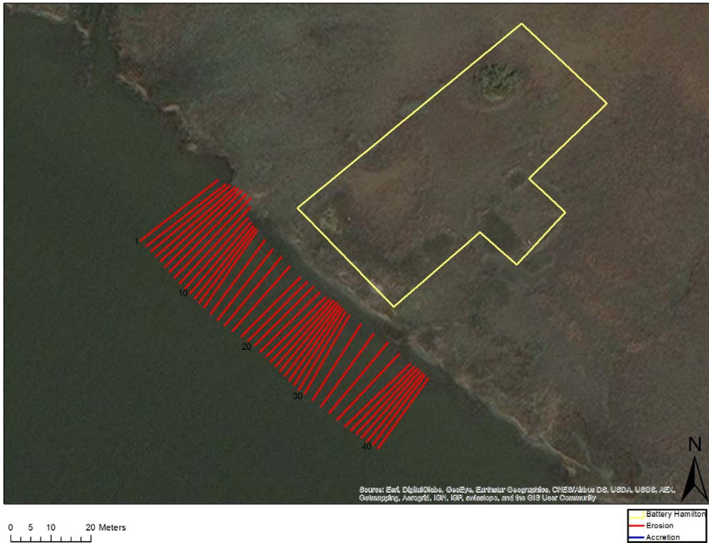
Figure 5: Character of shoreline change at Battery Hamilton. Red indicates erosion and blue indicates accretion. Length of line shows distance of shoreline movement from 1933 to 2013.
