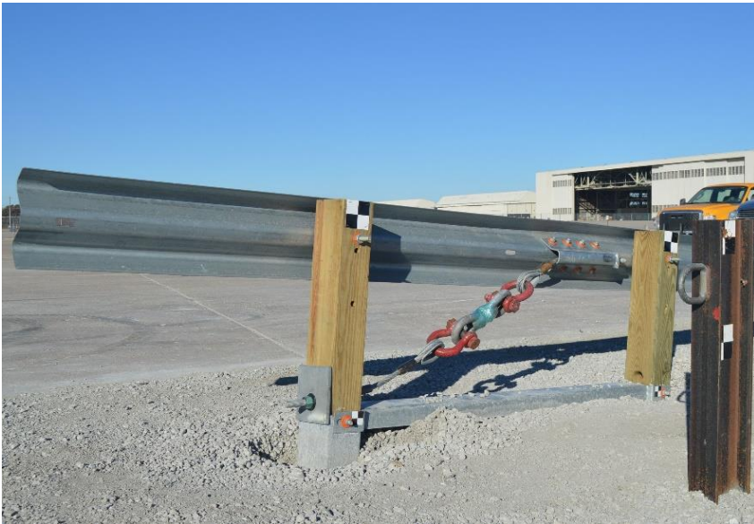
Figure 44. Upstream End Anchor Movement, Test No. GAA-1
