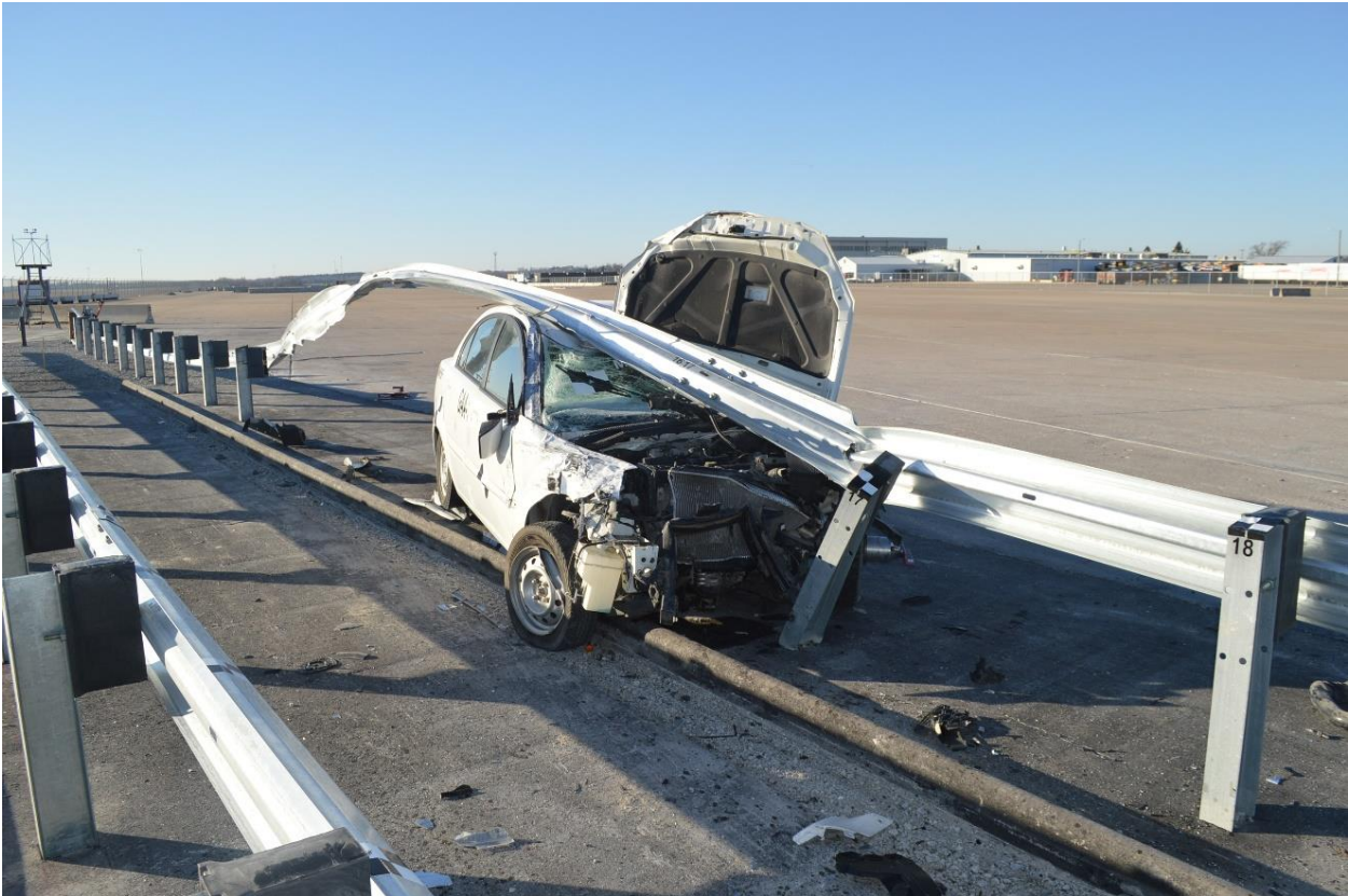
Figure 35. Vehicle Final Position and Trajectory Marks, Test No. GAA-1
