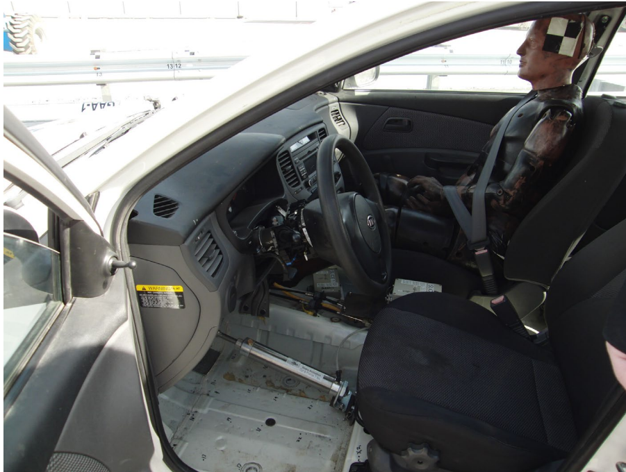
FIGURE 8 Simulated Occupant in Test Vehicle for GAA-1, TL 3-10
