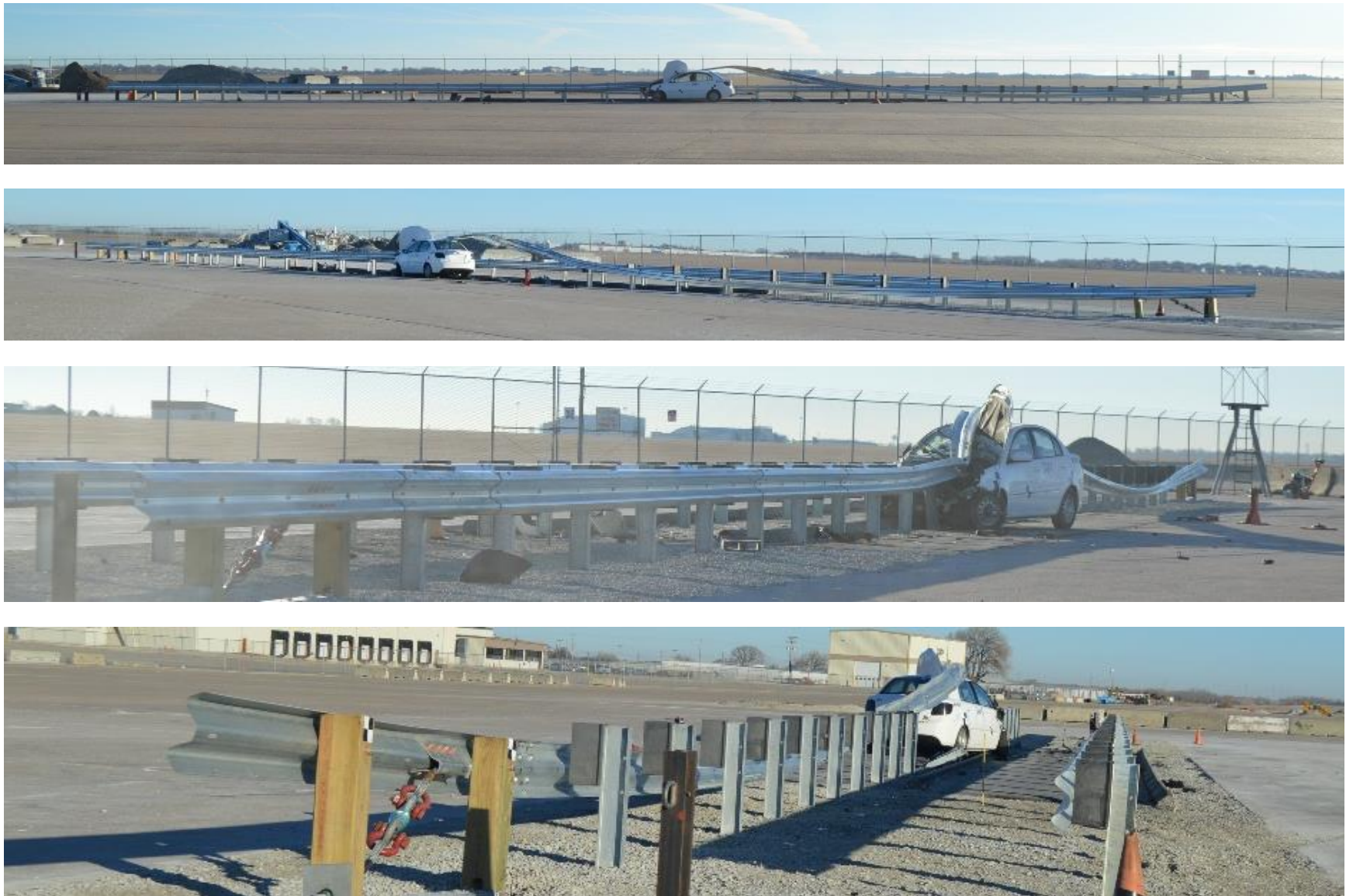
Figure 37. System Damage, Test No. GAA-1
