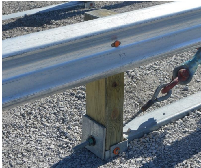
Figure 46. Post Nos. 28 and 29, Downstream End Anchorage, Test No. GAA-1
