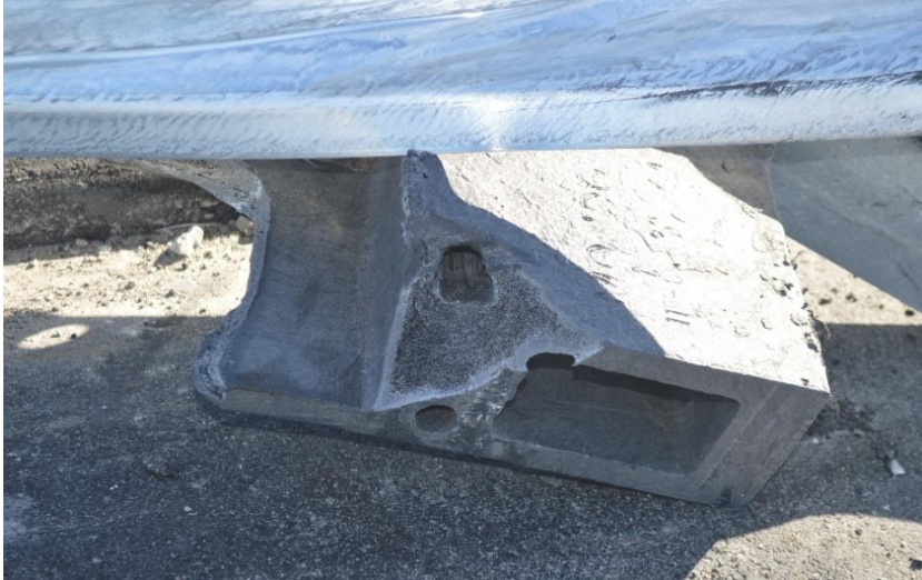
Figure 41. Post No. 13 Damage, Test No. GAA-1
