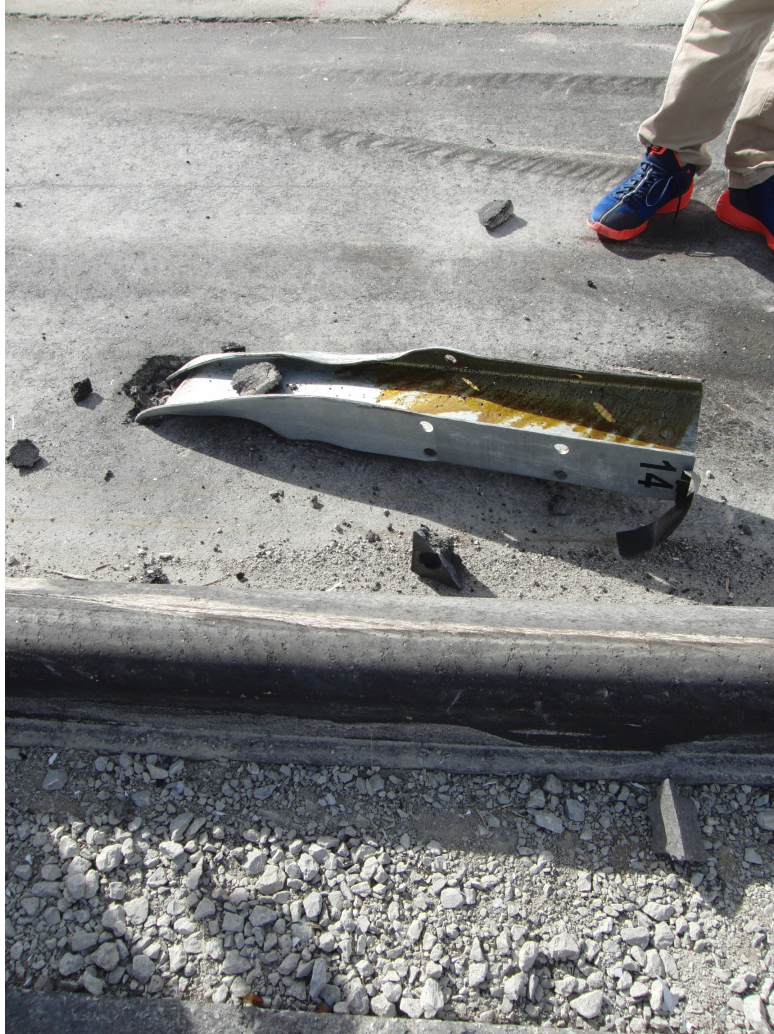
FIGURE 10 Buckled Post from Test GAA-1
