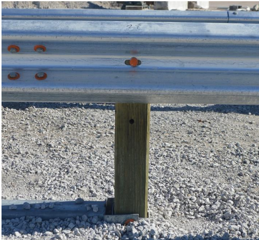
Figure 45. Downstream End Anchorage Movement, Test No. GAA-1
