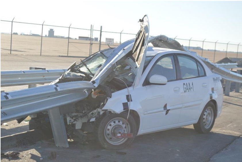
Figure 36. Vehicle Final Position, Test No. GAA-1
