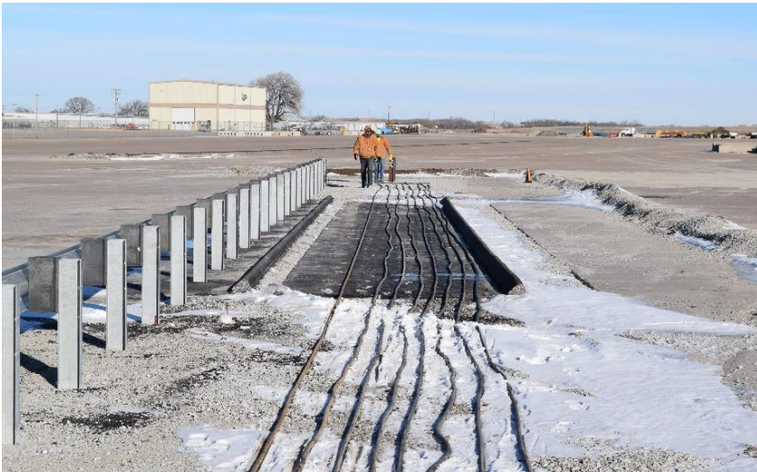
Figure 19. Test Construction – Soil and Asphalt Heating, Test No. GAA-1
