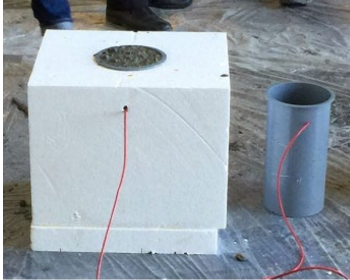
Figure 6. The insulated (left) and uninsulated (right) cylinders
