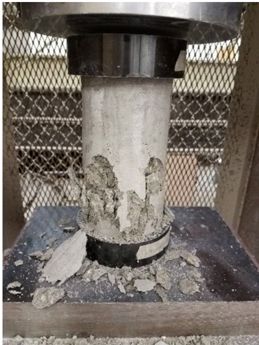
Figure 4. A scene of the compressive strength test
