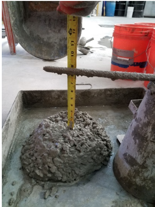
Figure 3. A slump test for the baseline concrete
