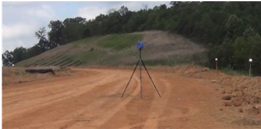
FIGURE 6 Laser scanning with sphere targets for resection
