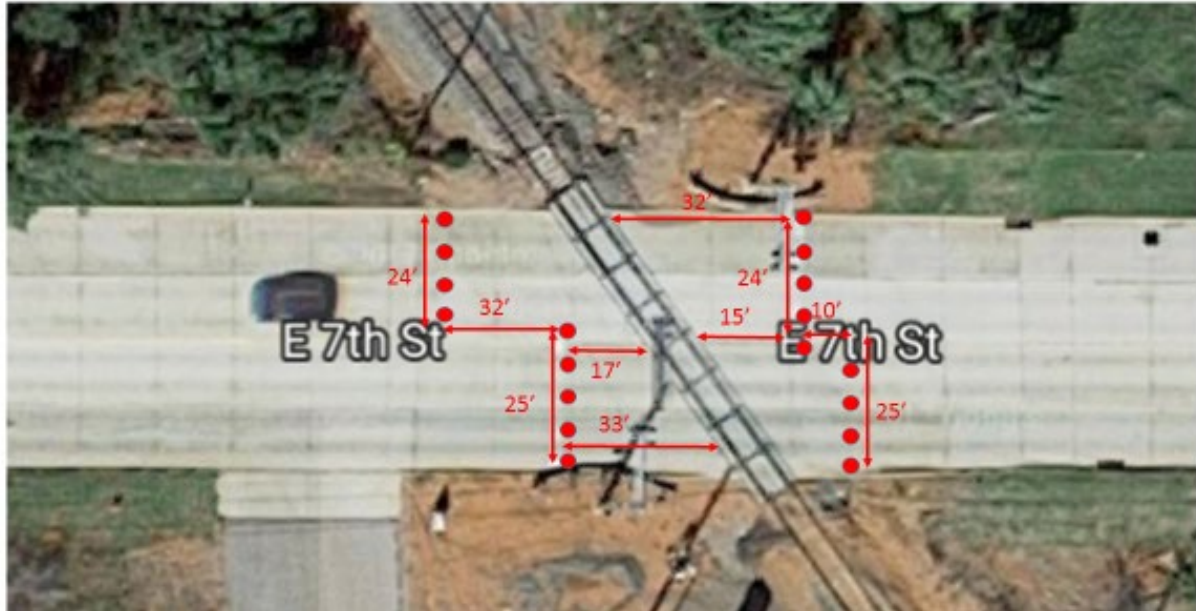
Figure 6 – Measurements of In-Pavement Light System in Elk City, Oklahoma (Source: Google Maps)
