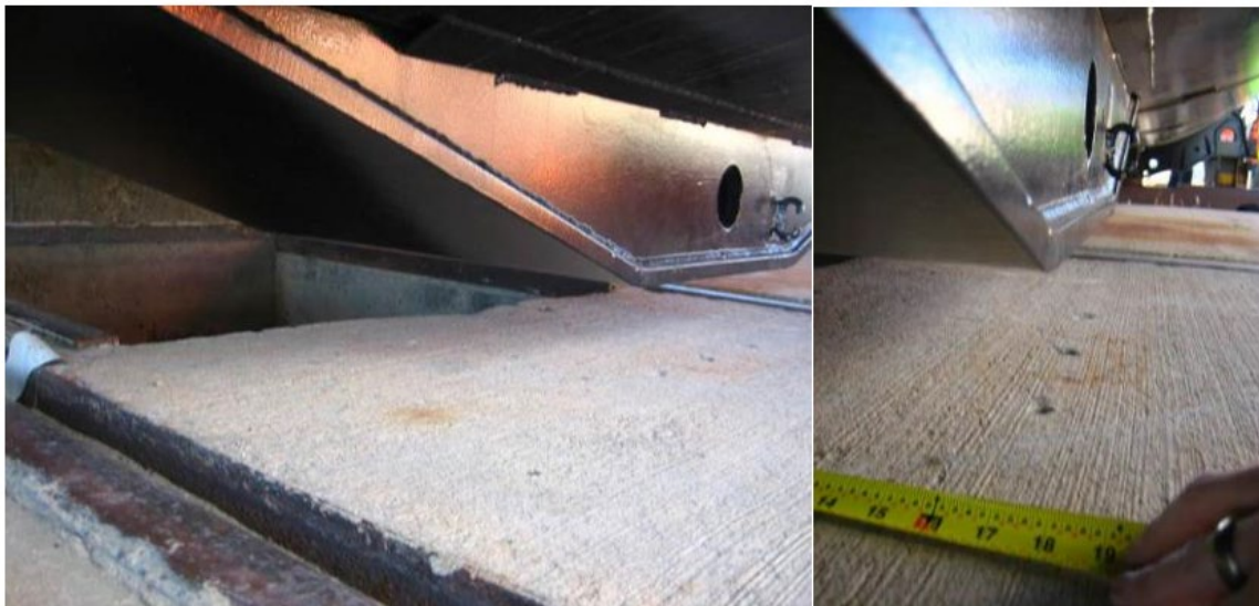
Figure 32. Pre-Test Positions of Bottom Protection and Pit (left) and Measurement from Leading Edge of Pit to Leading Edge of Bottom Protection (right)
