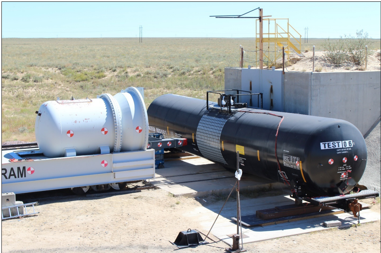
Figure 4. Target Tank Mounted on Support Skids
