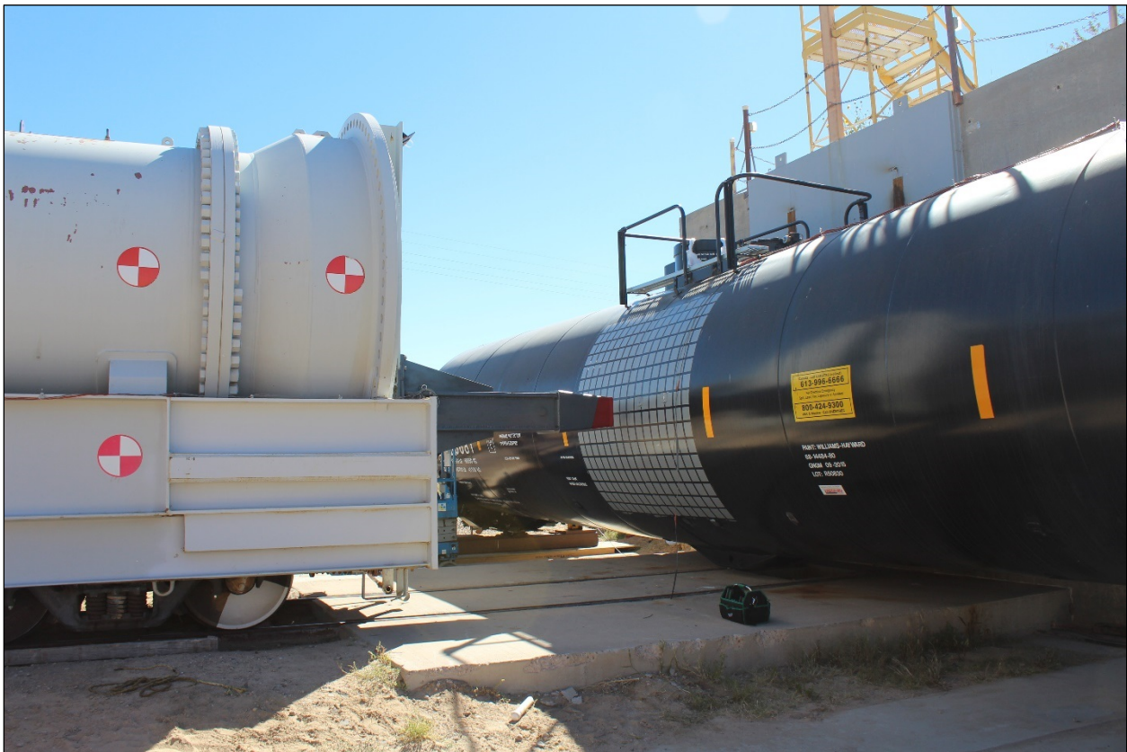
Figure 9. Ram Arm with 12-Inch by 12-Inch Indenter Aligned with Center of the Tank Car
