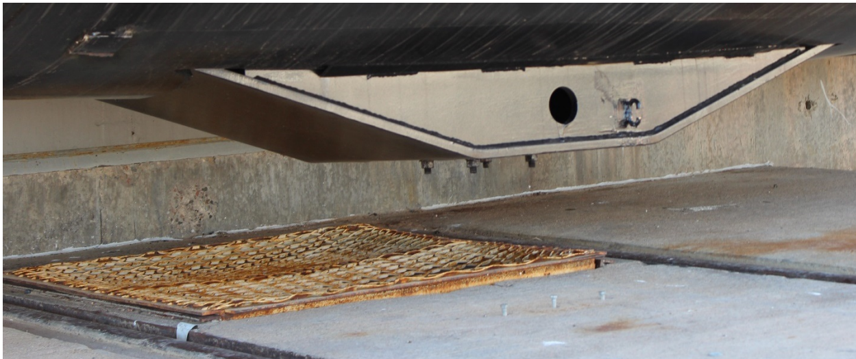
Figure 6. Tank Car's Bottom Valve Protection Structure
