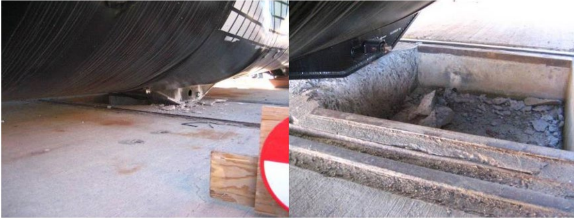
Figure 33. Post-Test Positions of Bottom Housing and Pit Viewed from Front (left) and Rear (right)
