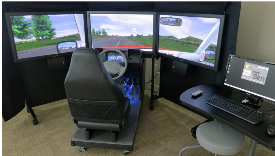
Figure 2 miniSim driving simulator with a quarter cab
