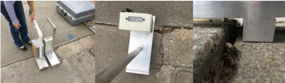
Figure 6-7 The controlled-environment testing using the original GFM and the new GFM prototype
