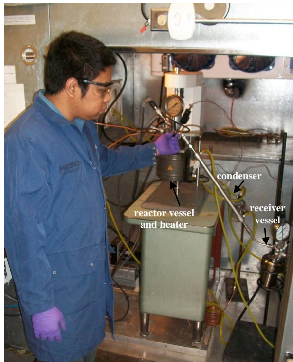
Figure 1: The modified continuous-flow reactor system (shown in the picture is PhD student Randy Maglinao).
