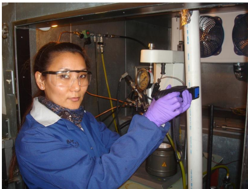
Figure 4: Undergraduate student Sonam Sherpa analyzing the gaseous products using Draeger gas detection tubes.
