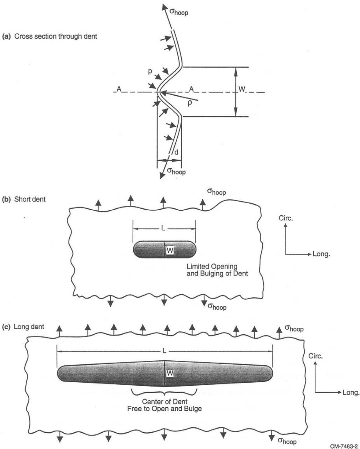
**Figure 2. Schematic of Dent in a Tank Car.**
