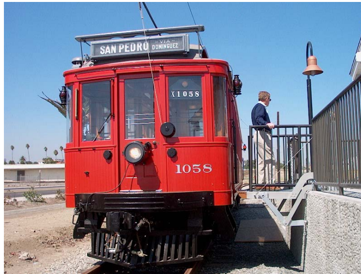
Figure 72: Red Car at Platform, Showing Retractable Extension
