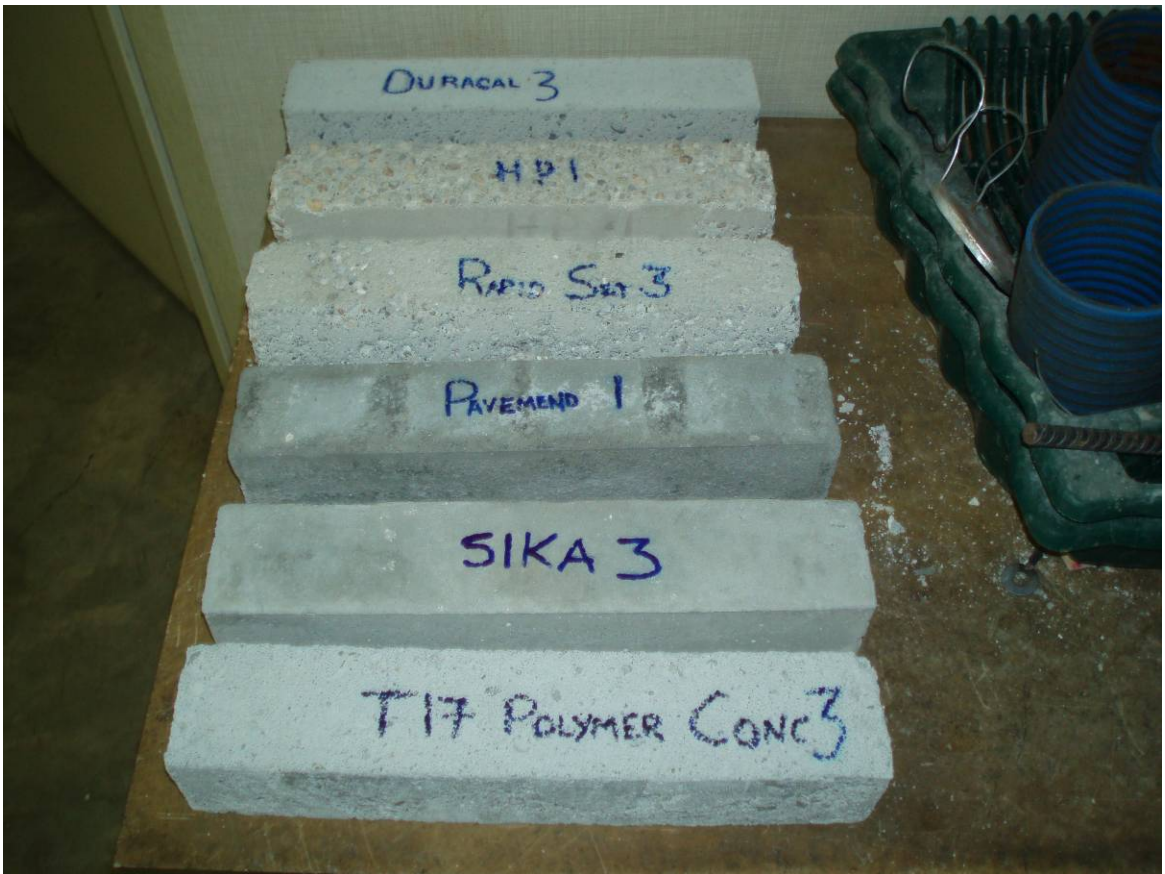
Figure A-1: Regular Water Freeze-Thaw Specimens
