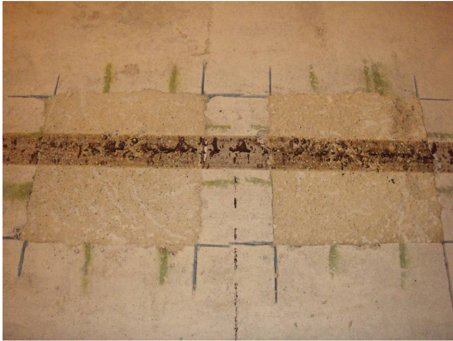
Figure 3-26: Repetitive Tire Loading – Rapid Set Patches
