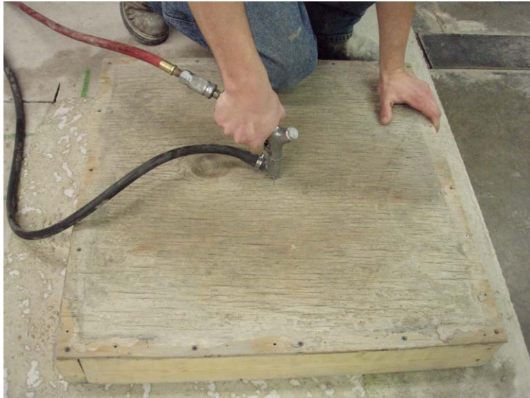
Figure 3-28: Sandblasting Specimen – ASTM C 418
