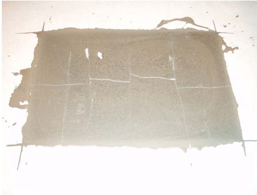
Figure B-7: Three-Point Loading – Pavemend 15.0 –Large, Deep
