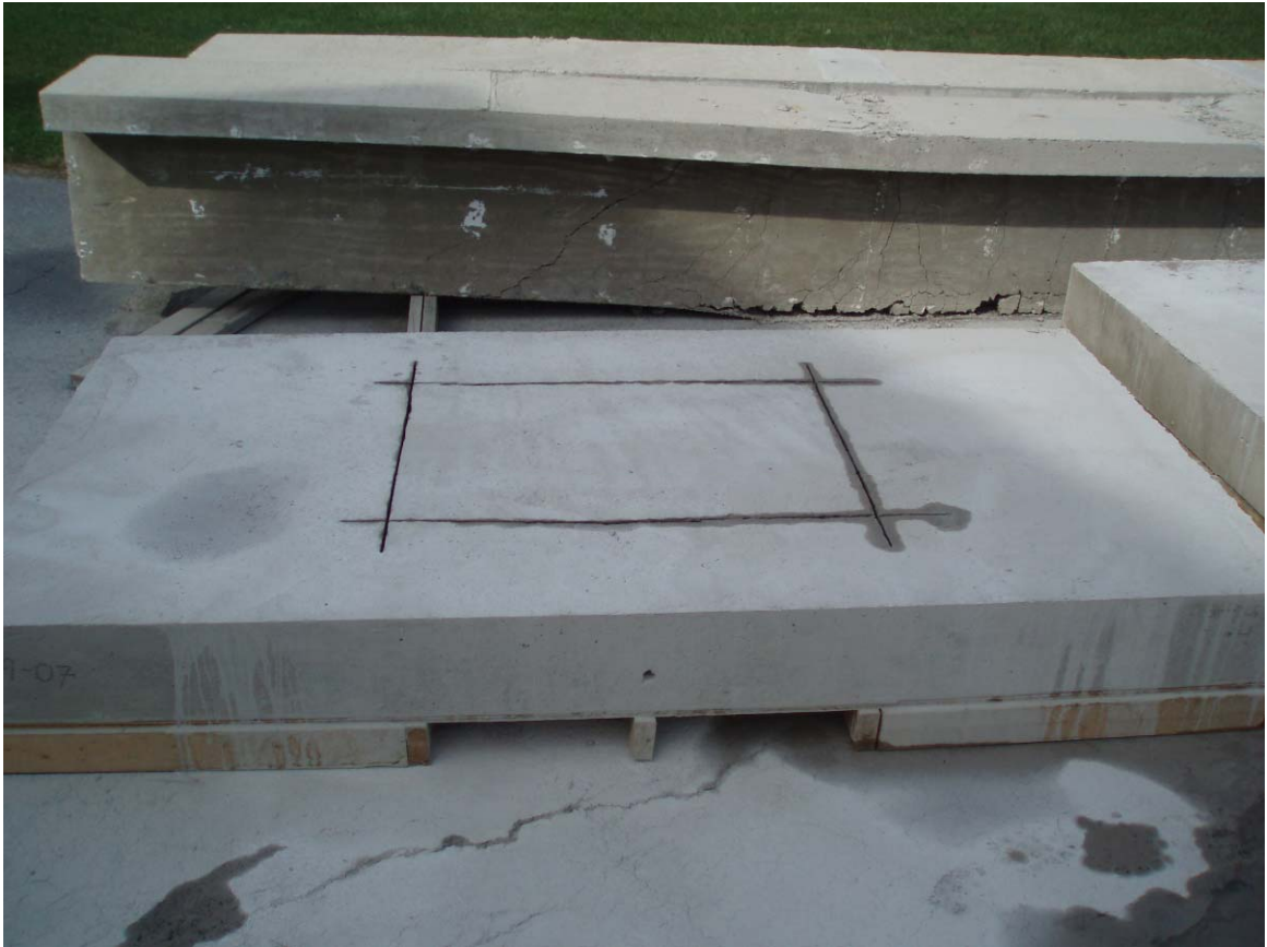
Figure 3-6: Saw-Cut Test Slab
