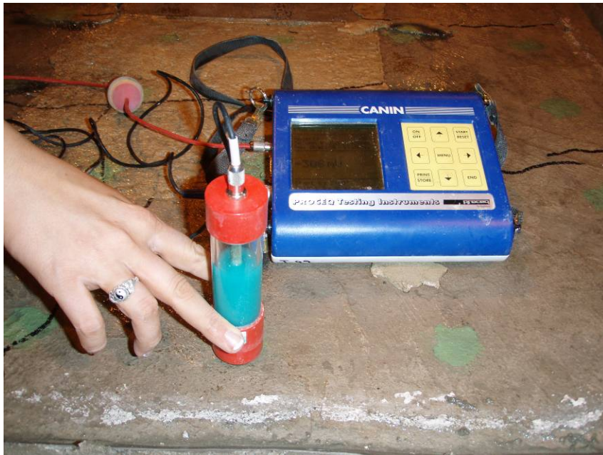
Figure 3-32: Half-Cell Potential Readings
