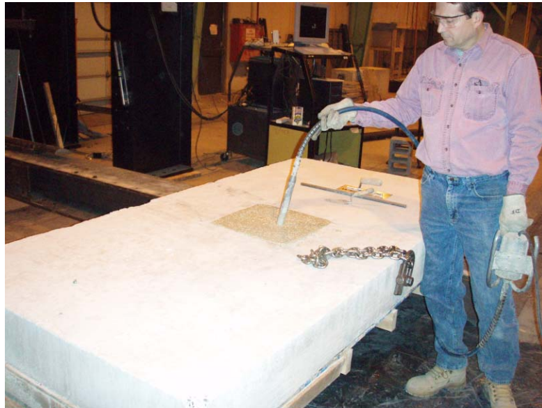
Figure 3-13: Vibrating Rapid Set
