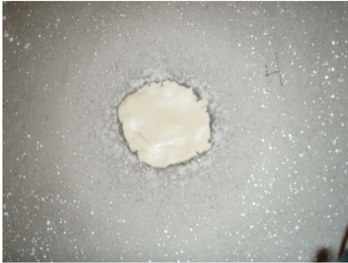
Figure 3-29: Sandblasted Hole Filled With Clay – ASTM C 418
