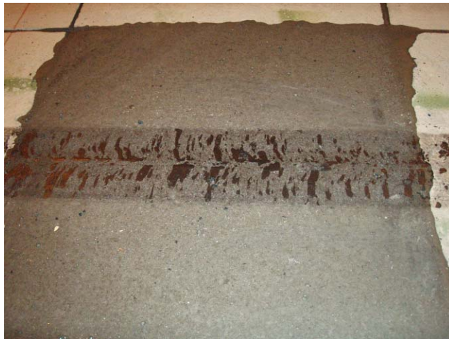
Figure B-9: Pavemend 15.0 Patch after Tire Load Simulation – Close-up 1
