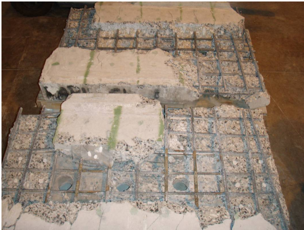
Figure 3-44: Slabs After Autopsy (Rapid Set on Top, Pavemend on Bottom)
