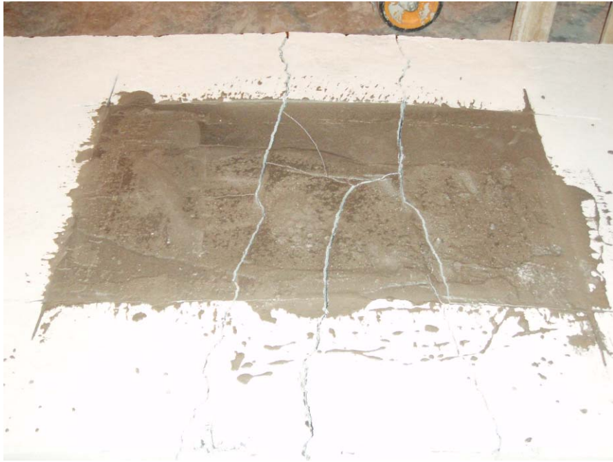
Figure B-3 : Three-Point Loading – Pavemend 15.0 – Large, Shallow
