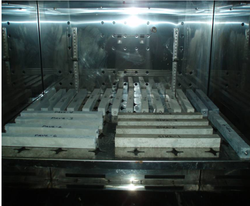
Figure 2-5: ASTM C 531 M (Specimens heated in oven)
