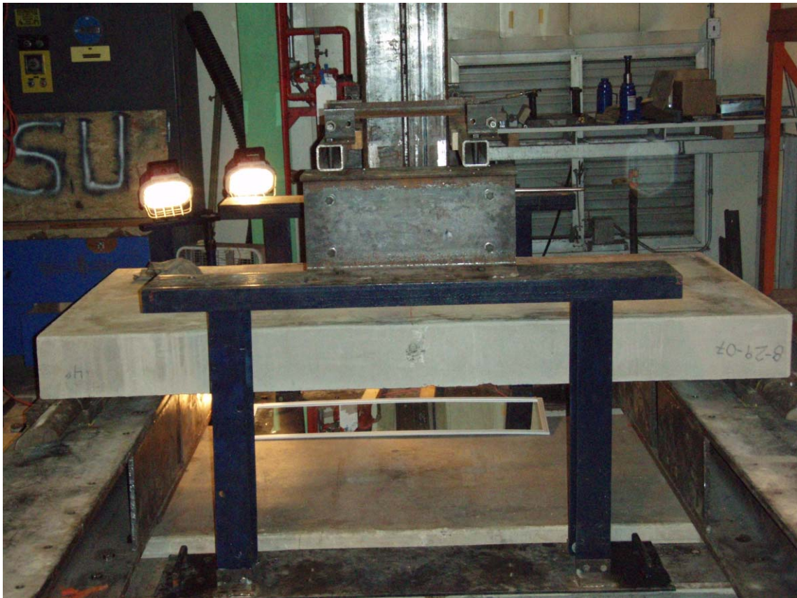
Figure 3-17: Slab Under Actuator
