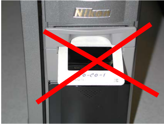
Figure 4 – Incorrect Insertion of Slide
