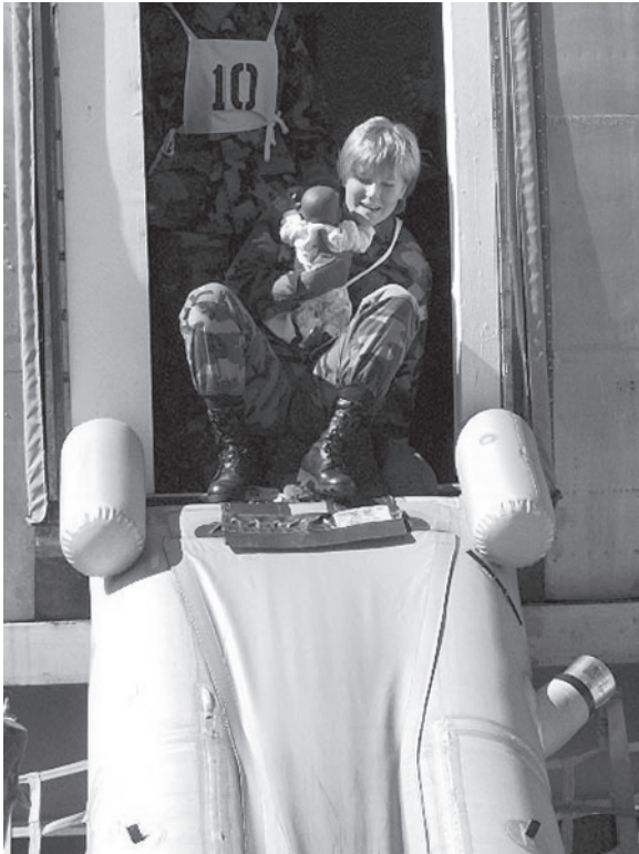
Figure 17. Infant carrier holds newborn dummy vertically with one hand while steadying herself with the other.
