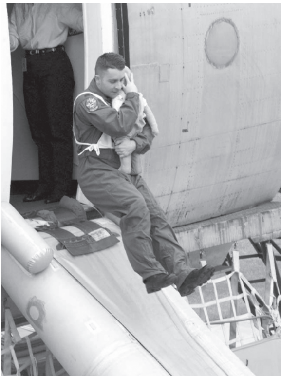
Figure 18. Infant carrier holds 6-month dummy vertically, supporting head, neck, and back, and jumps to board slide.
