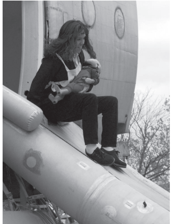
Figure 14. Infant carrier holds 6-month dummy horizontally and sits on slide to board.
