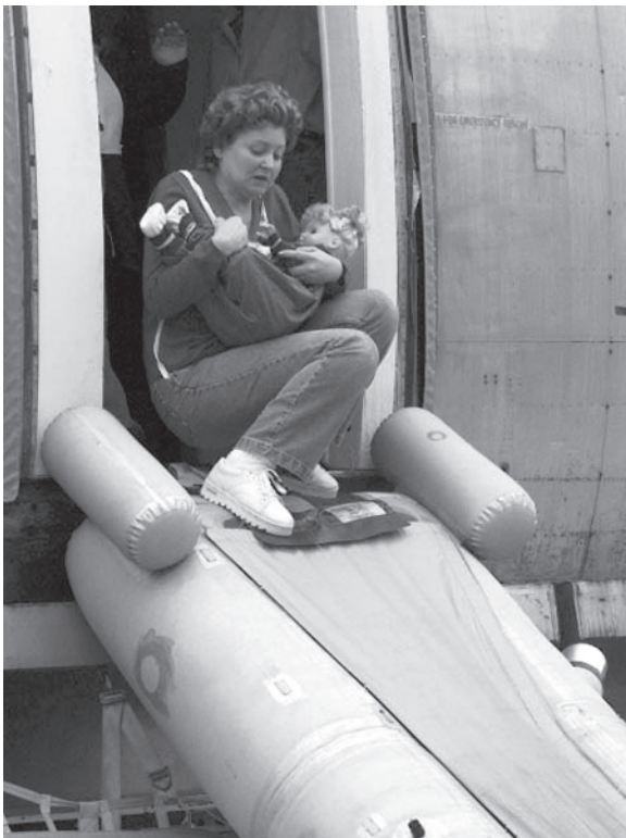
Figure 15. Infant carrier holds 24-month dummy horizontally and sits on slide to board.
