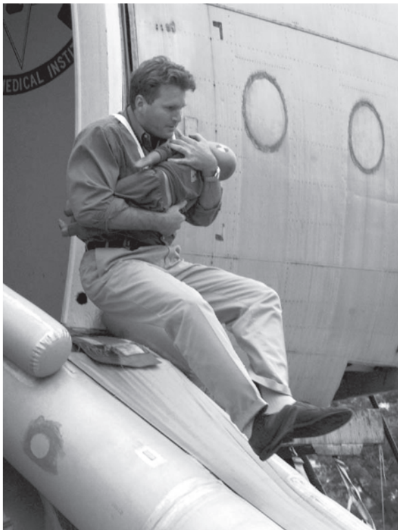
Figure 11. Infant carrier hold 18-month dummy horizontally and jumps onto slide.
