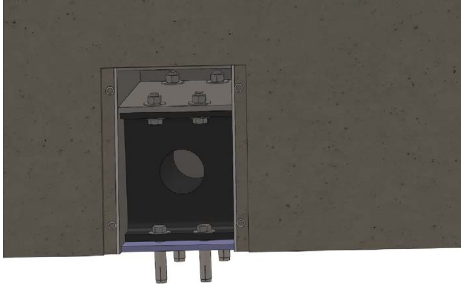
Figure 2.24. Close-up Details of Single Rubber Fender Inserted within the Concrete Barrier.
