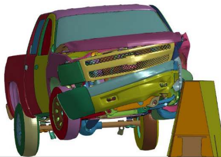
Figure 4.20. Vehicle Interaction with Barrier (Four 40-ft Segments – Three Rubber Fenders).
