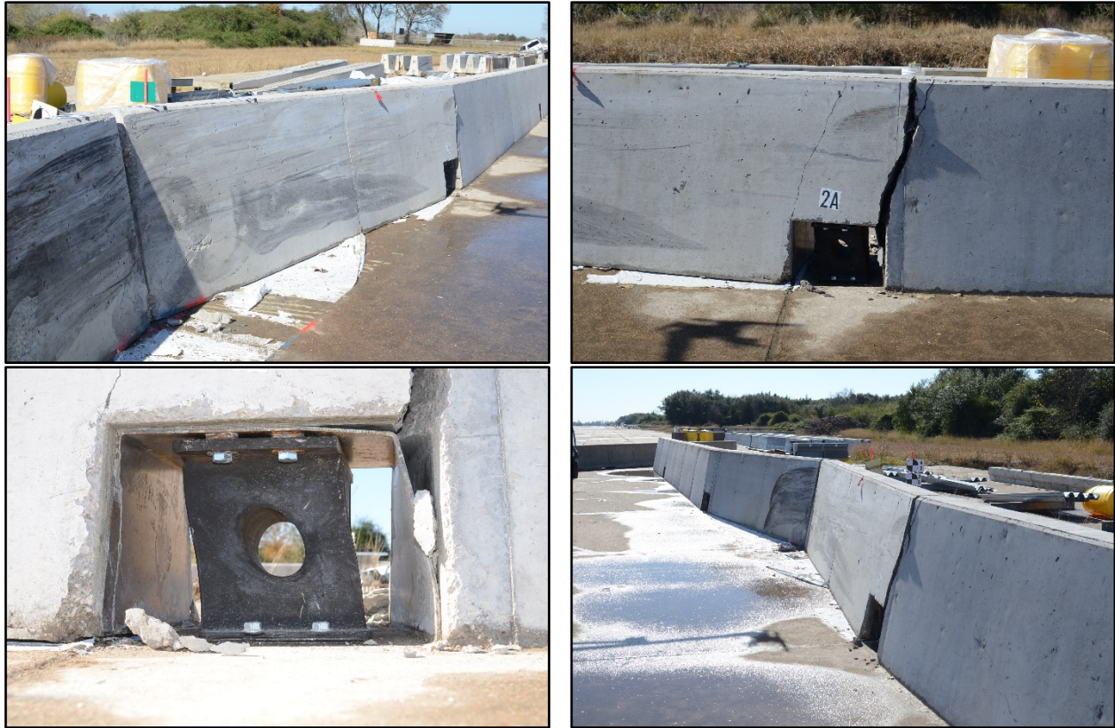
Figure 10.5. Damage to Barrier #2 after Test No. 468958-2.
