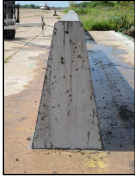
Figure 5.38. Right End and Field Side of Barrier after Test No. 468957-B9.
