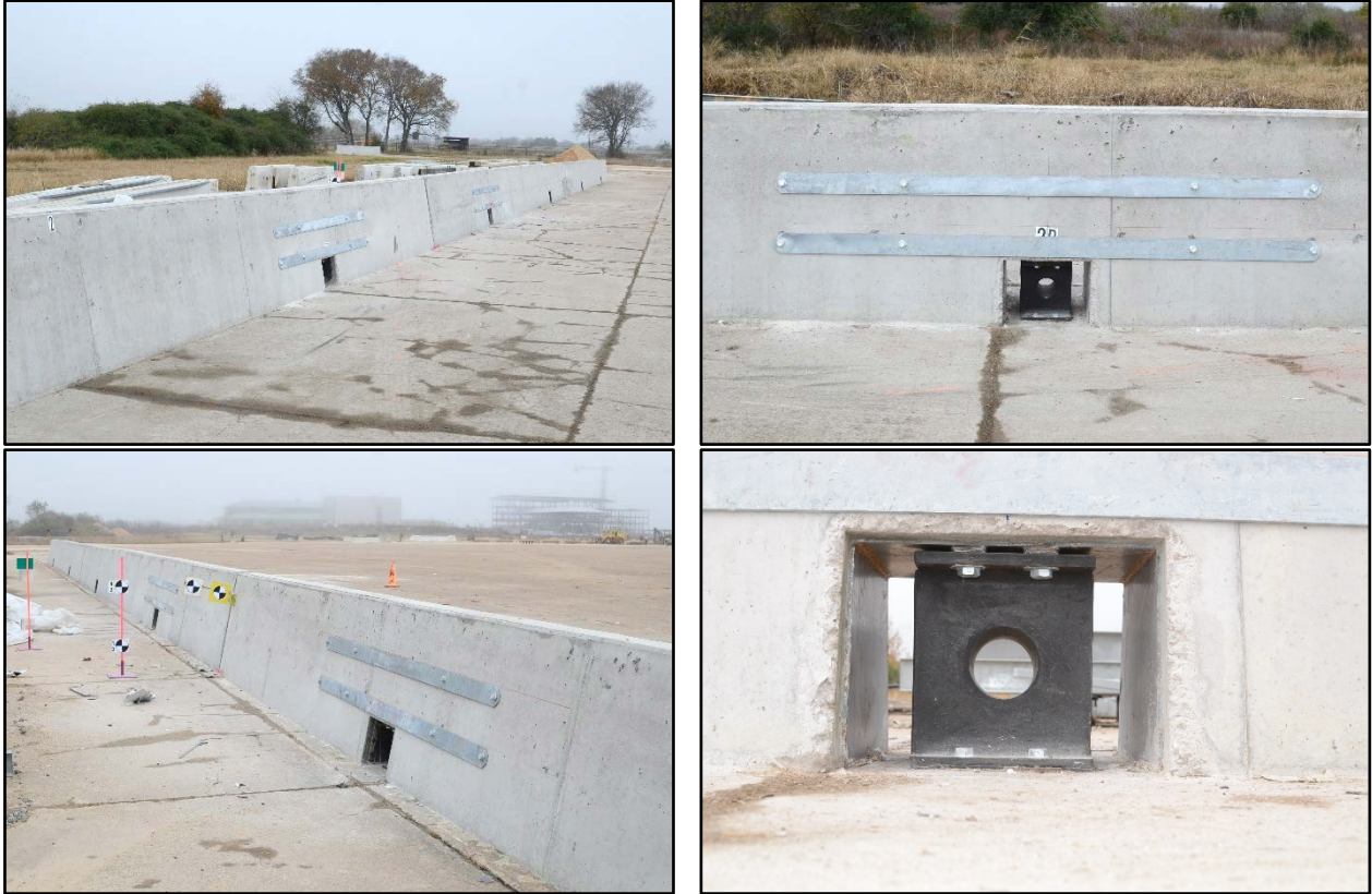
Figure 6.3. Straps Used on TxDOT Rubber Mounted Single Slope Barrier prior to MASH Test 4-12.
