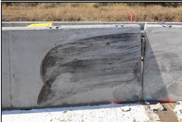
Figure 10.4. Damage to Barrier #1 after Test No. 468958-2.
