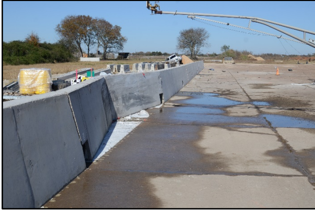
Figure 10.3. TxDOT Rubber Mounted Single Slope Barrier after Test No. 468958-2.
