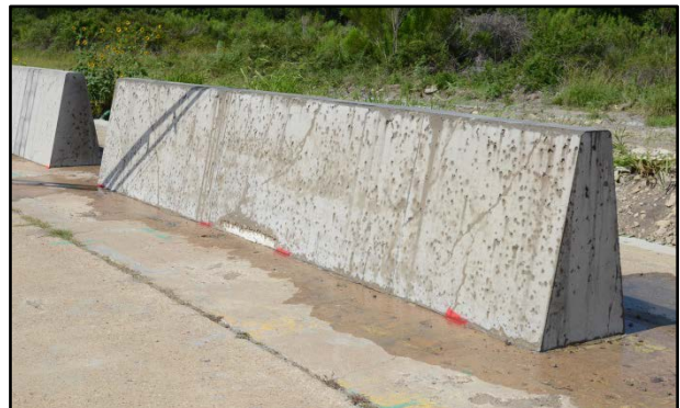
Figure 5.39. Left End and Traffic Side of Barrier after Test No. 468957-B9.
