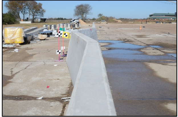
Figure 10.3. TxDOT Rubber Mounted Single Slope Barrier after Test No. 468958-2.
