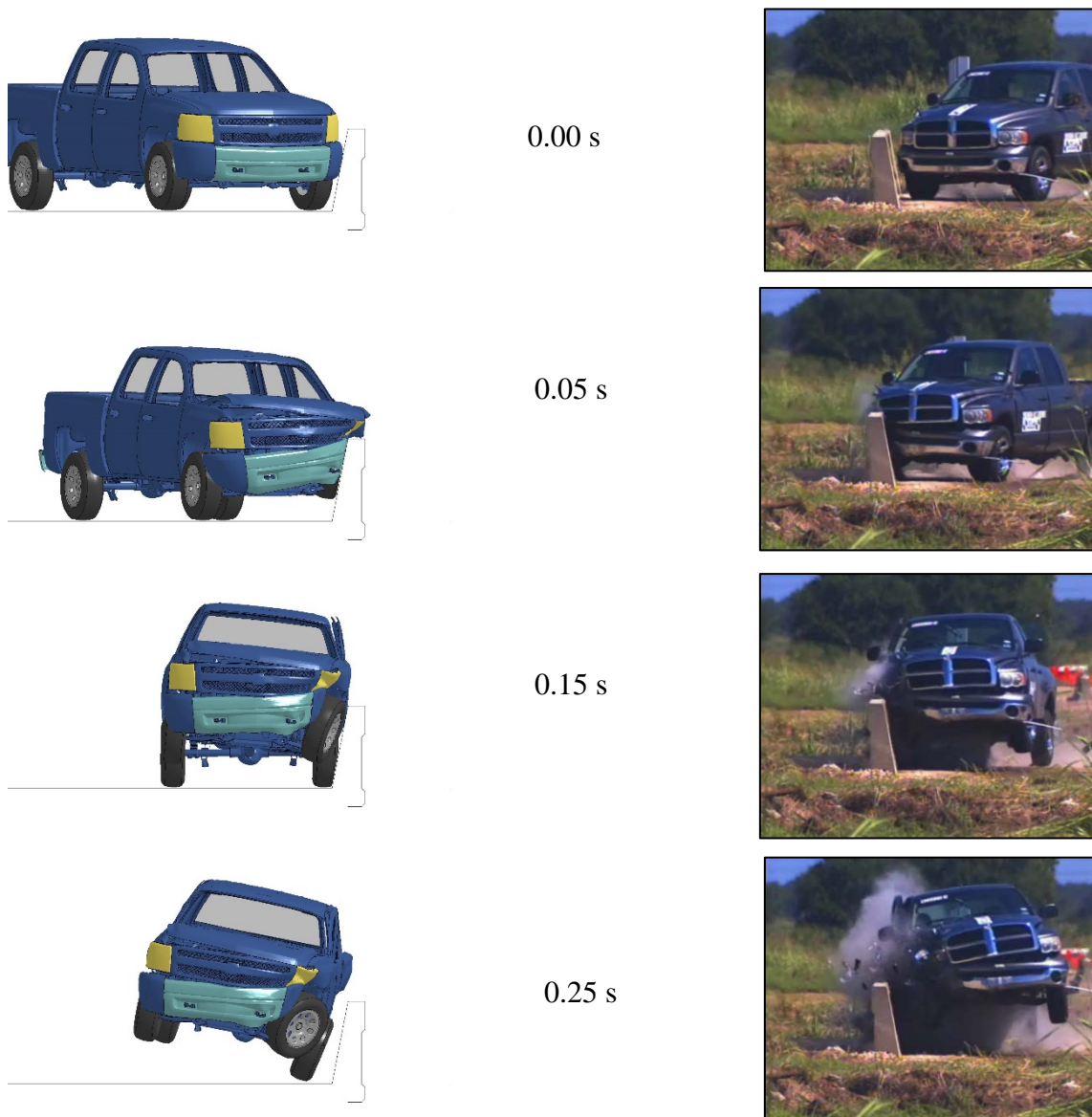
Figure 2.6. Sequential Comparison of Pan Form Test (Right) and Simulation (Left) under MASH Test 3-11 Impact Conditions.
