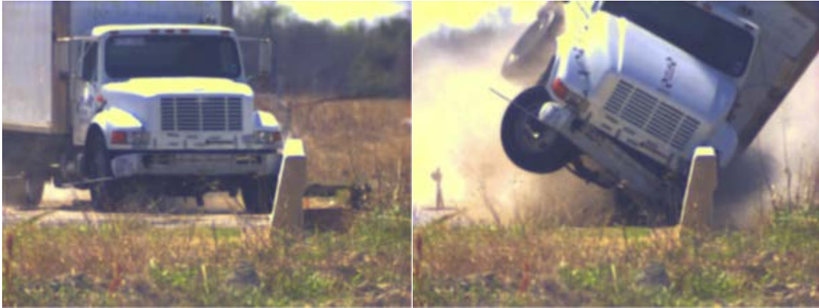
Figure 2.3. Sequences Showing SUT Impacting a 36-inch Tall Texas SSTR.
