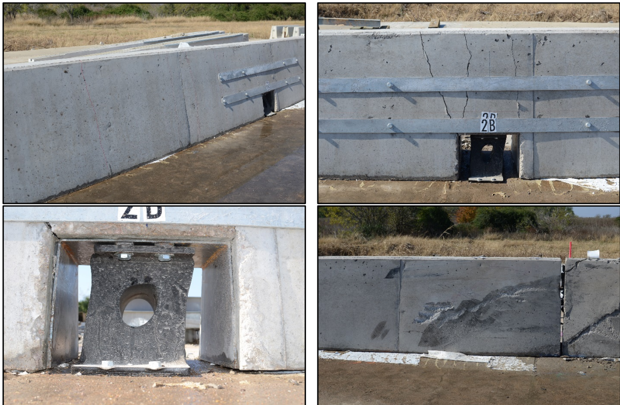
Figure 11.4. Damage to Barrier #2 after Test No. 468958-3.
