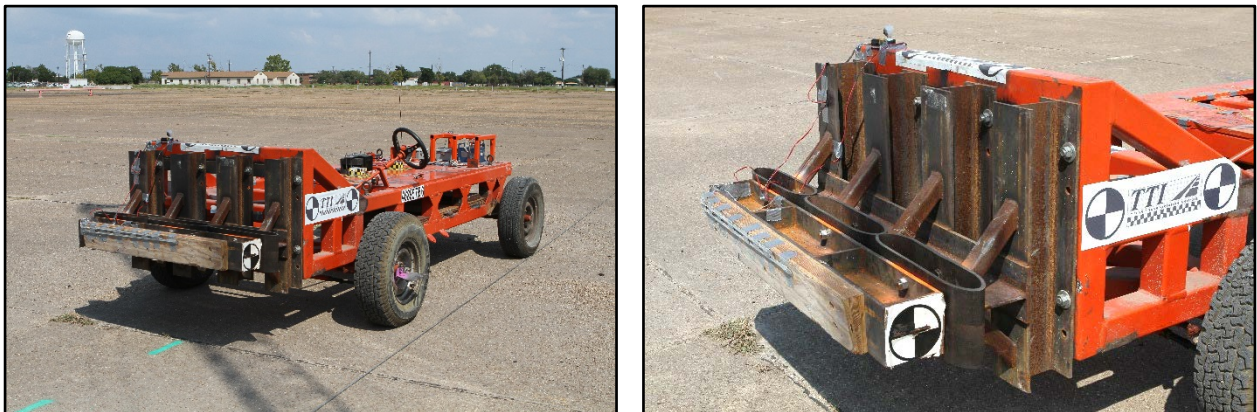
Figure 5.24. Bogie Vehicle after Test No. 468957-B7.
