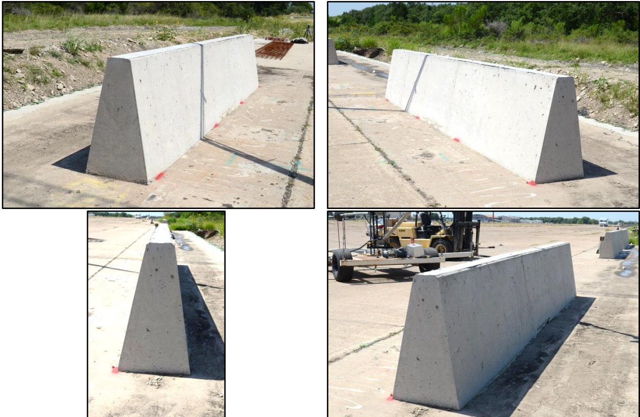
Figure 4.46. CR10F-Gnet Mix Concrete Barrier before Test No. 468957-B10.
