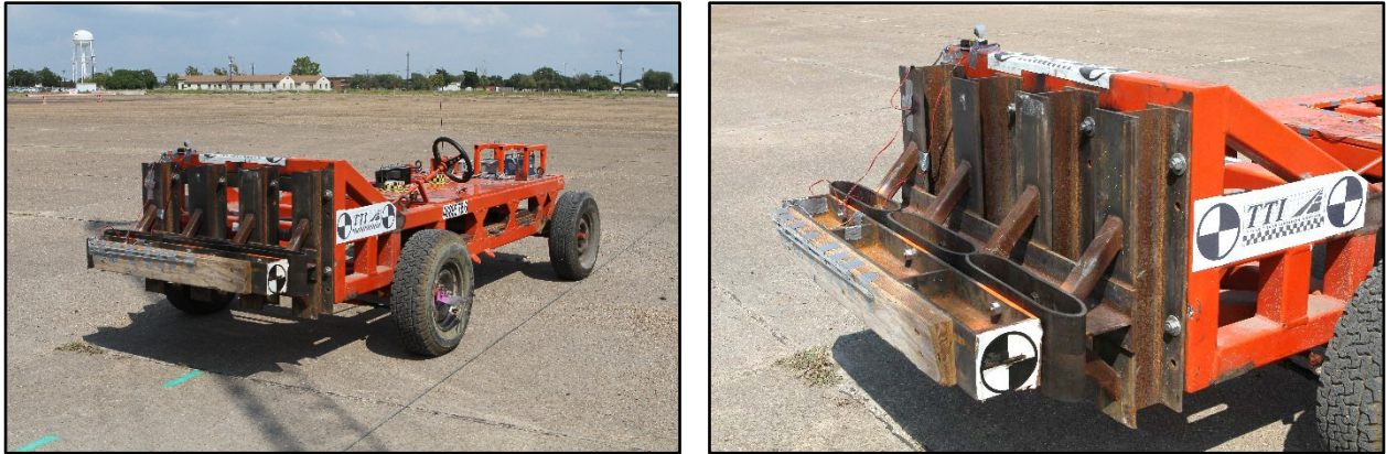
Figure 5.18. Bogie Vehicle after Test No. 468957-B6.
