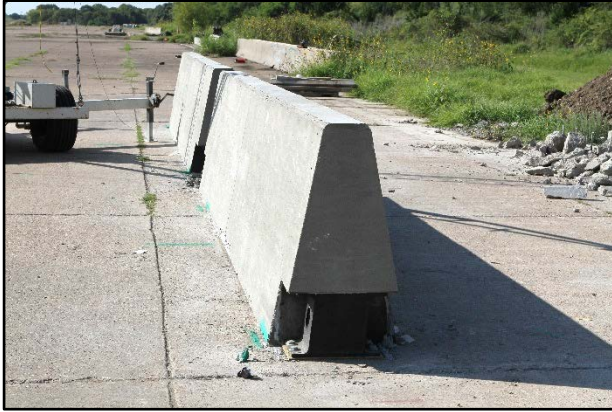
Figure 5.3. Right Traffic Side of Barrier after Test No. 468957-B4.
