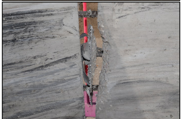
Figure 10.4. Damage to Barrier #1 after Test No. 468958-2.
