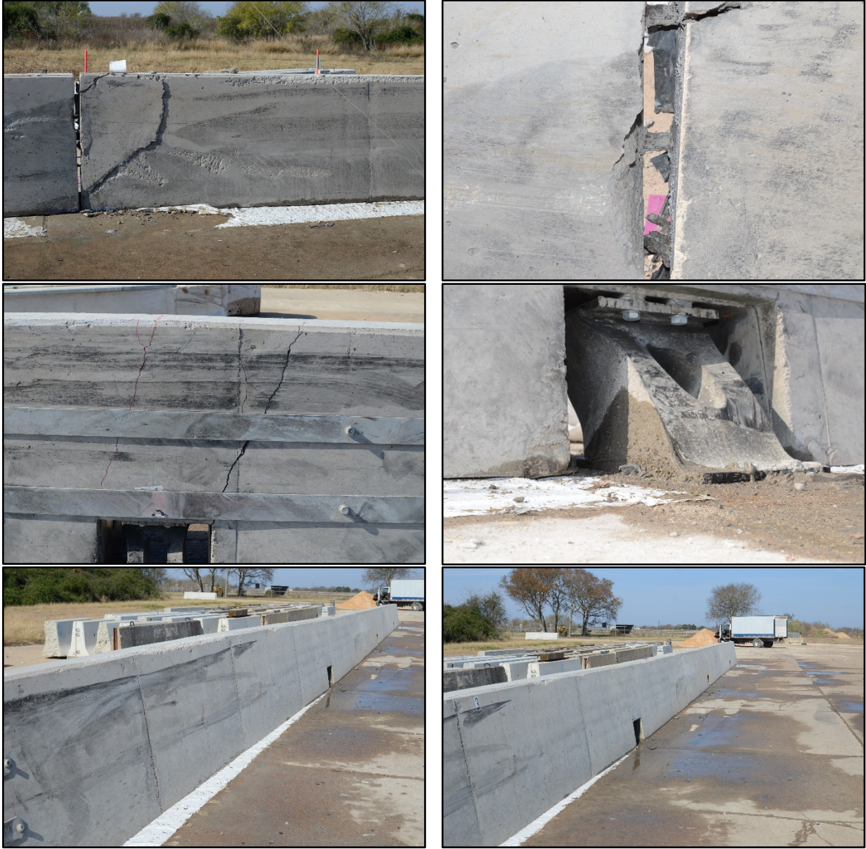
Figure 11.5. Damage to Barrier #3 after Test No. 468958-3.
