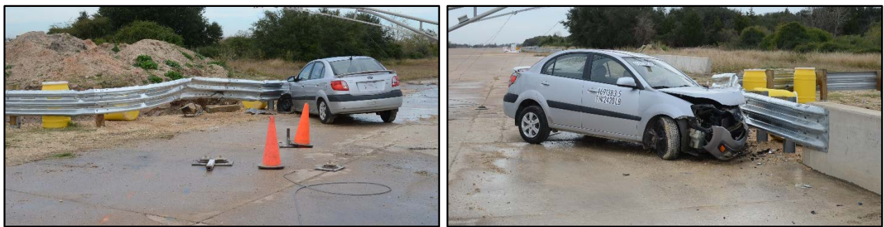
Figure 11.3. TxDOT Low-Speed Short Radius Guardrail/Test Vehicle after Test No. 469138-3-5.
