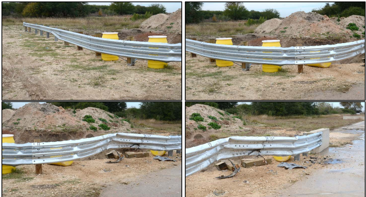
Figure 11.4. TxDOT Low-Speed Short Radius Guardrail after Test No. 469138-3-5.
