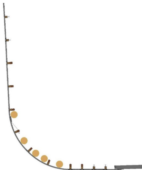
Figure 3.15. Tension Cable and Five 700-lb Sand Drums.
