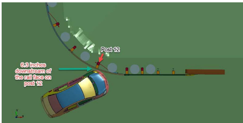
Figure 5.5. Target CIP for Modified MASH Test 2-34 on the TxDOT Low-Speed Short Radius Guardrail Treatment.
