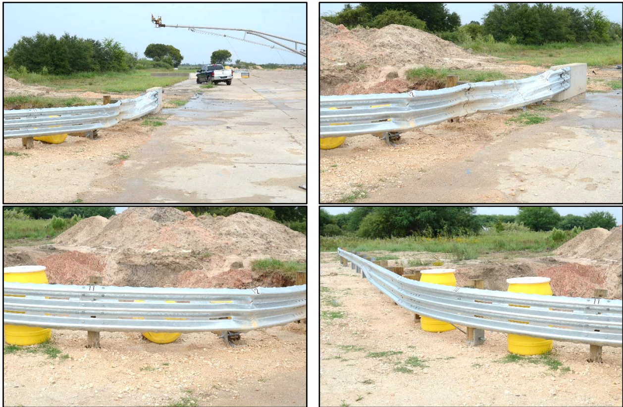
Figure 10.3. TxDOT Low-Speed Short Radius Guardrail Treatment after Test No. 469138-3-4.
