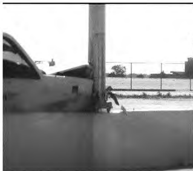
Figure 34. Fender Impact with a Rigid Pole [11]
