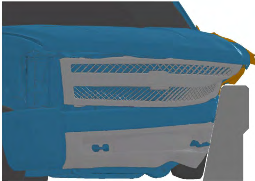
Figure 33. Fender Protrusion Over the Barrier (Note: Fender is orange for distinction)
