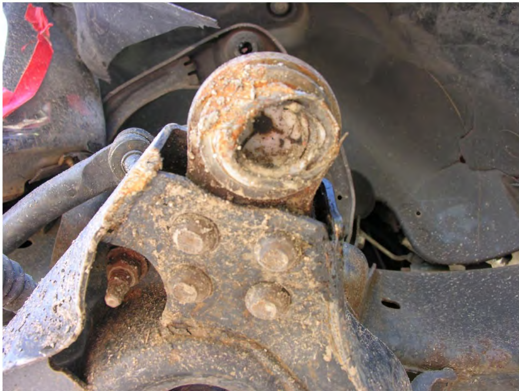
Figure 9. Lower Control Arm Damage, Test No. PCMB-1
