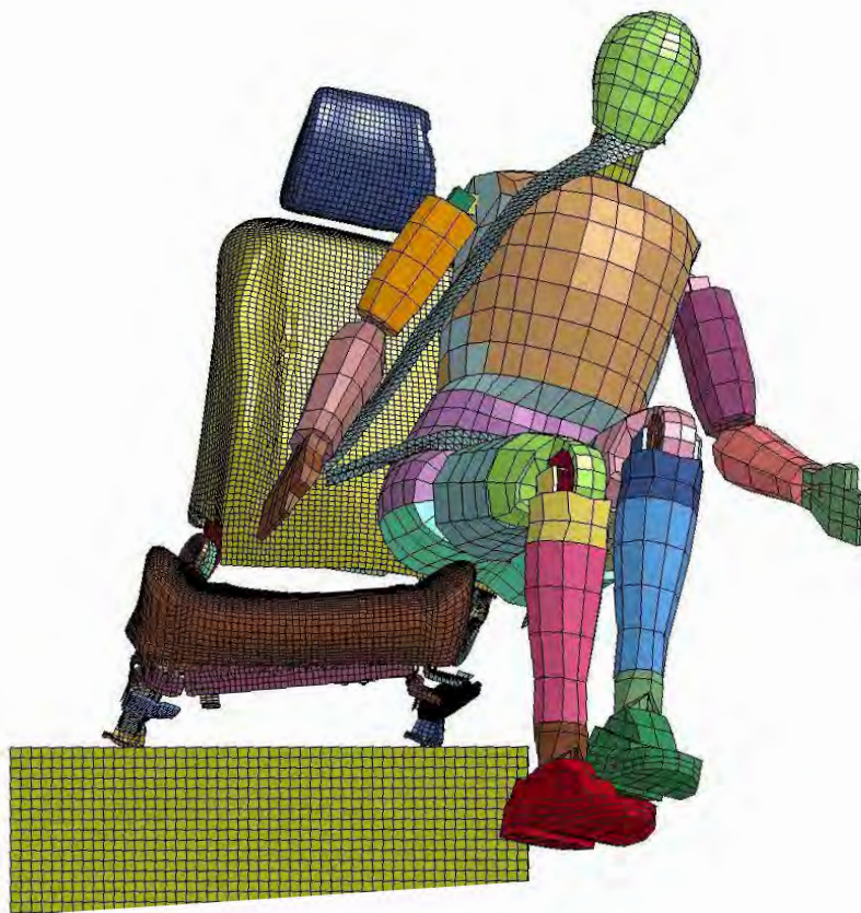
Figure 79. Seat, Seatbelt, and Dummy when Accelerated to the Right
