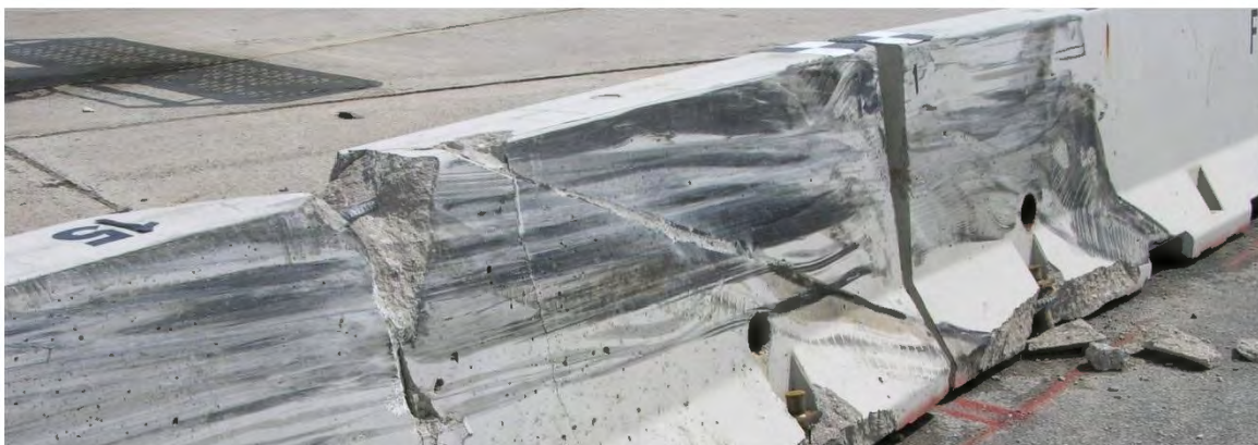
b. Contact Marks from Test No. FTB-2
