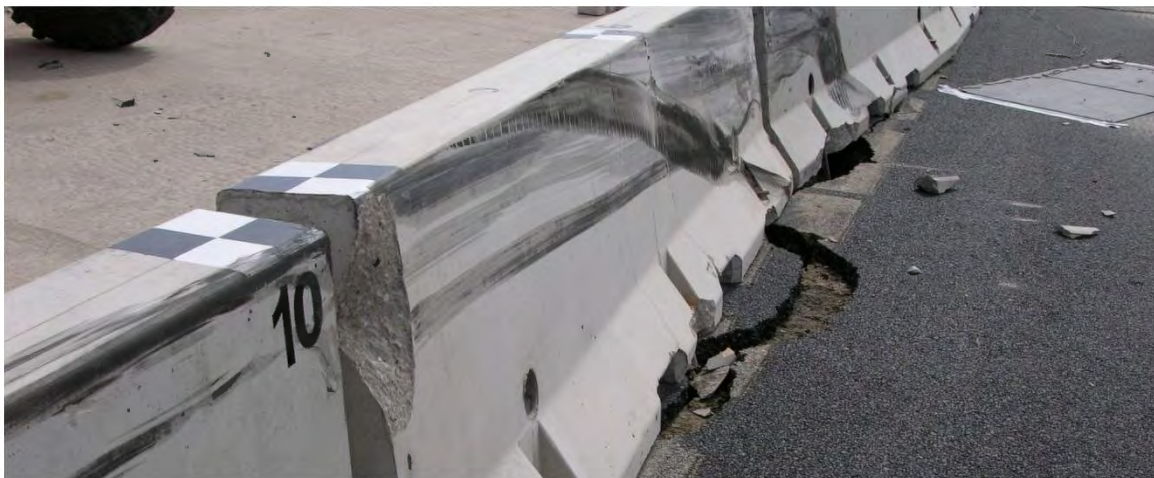
a. Contact Marks from Test No. FTB-1
