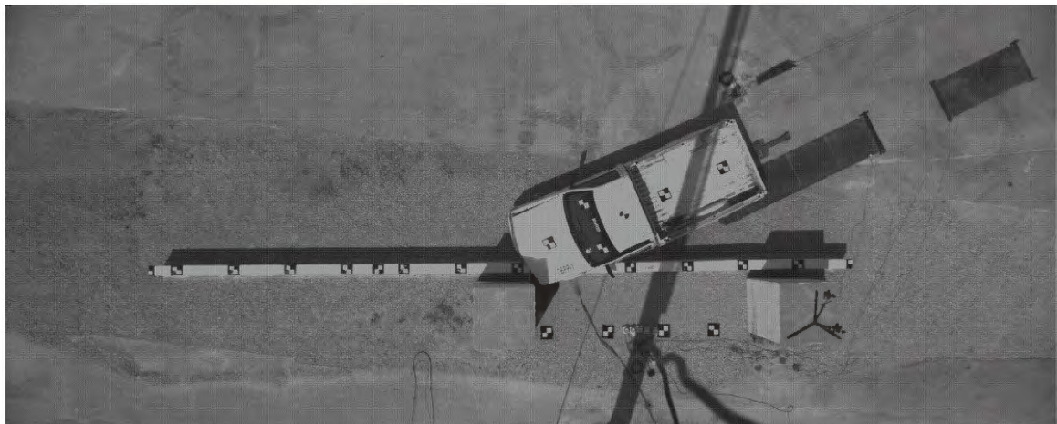
Figure 4. Impacting a Bridge Pier in the ZOI
