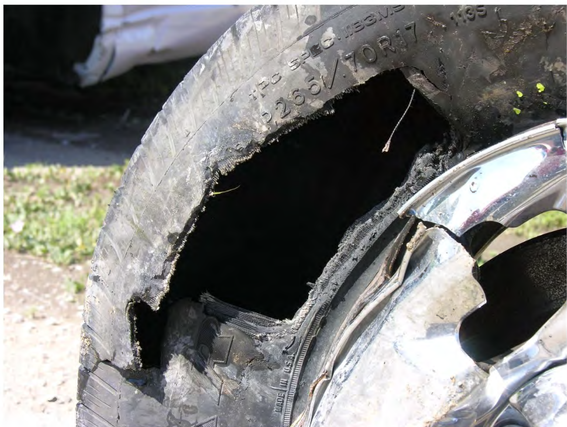
Figure 8. Outside of Wheel Damage, Test No. PCMB-1
