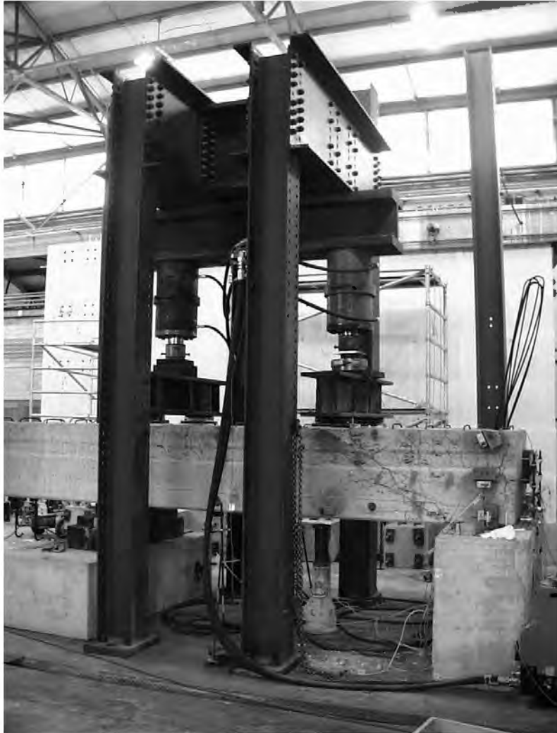
Figure 3.3 Loading setup for shear-dominated fatigue specimens
