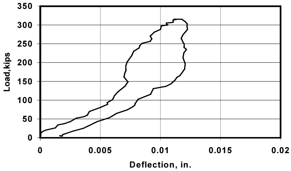
BG3N - North Bearing Pad (East Web)
