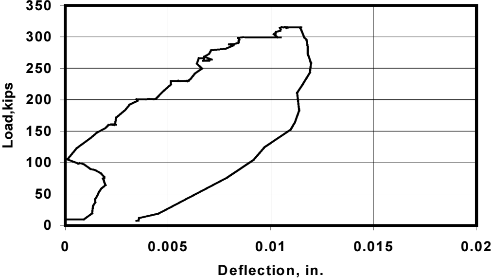
BG3N - North Bearing Pad (East Web)
