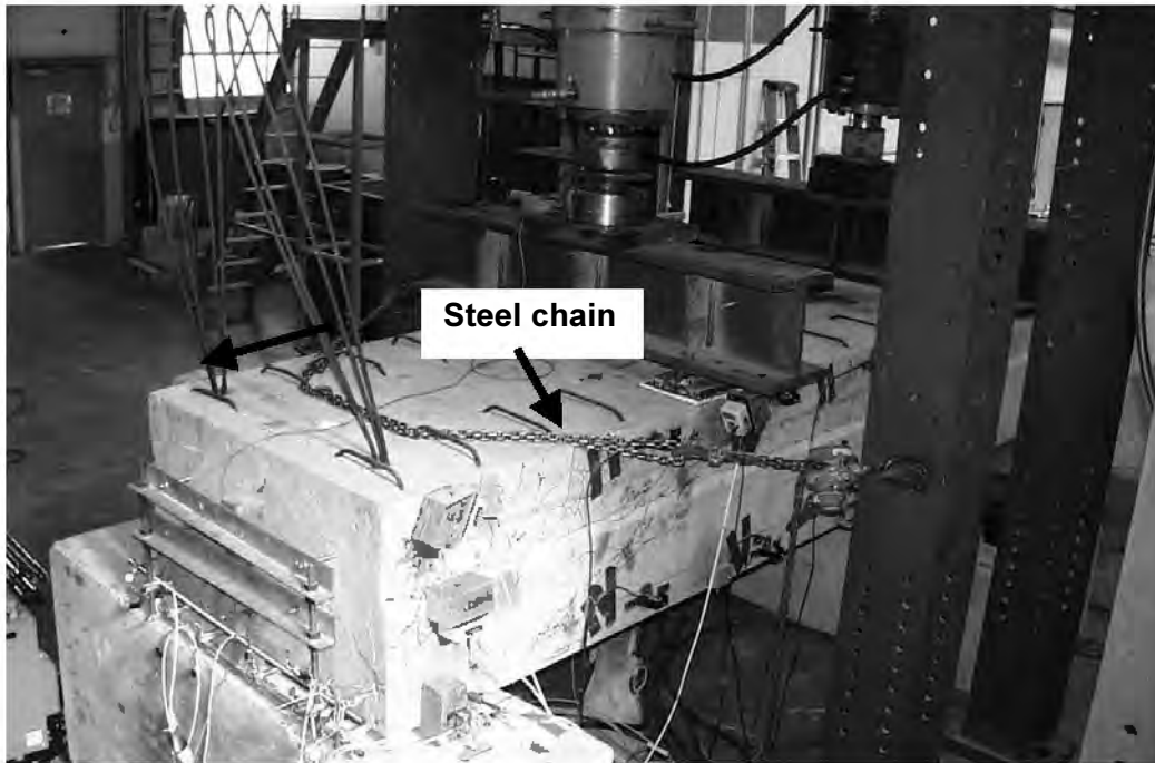
Figure 4.9 Longitudinal girder restraint placed after 10,000 load cycles
