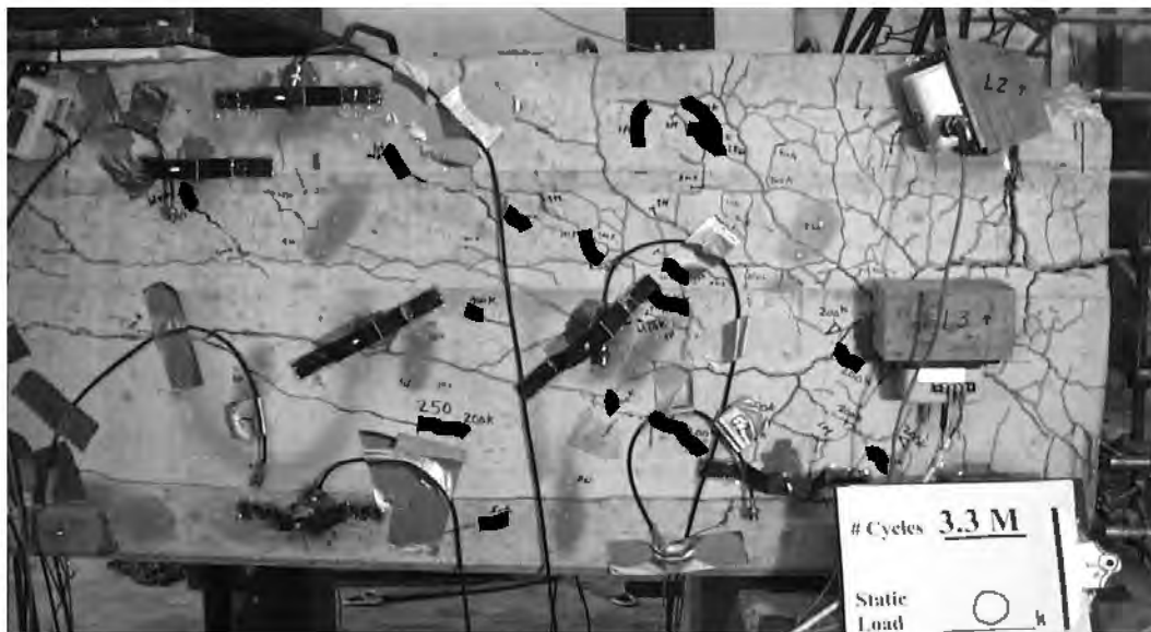
Figure 4.26 Shear-induced cracks in the west web of BG3S after 3,328,600 load cycles
