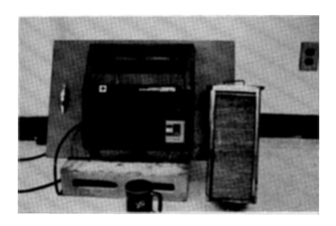
FIG. 16 The Lossnay [10] air-to-air residential heat exchanger manufactured by Mitsubishi Electric Co. in Japan. The unit is self contained including supply and exhaust fans. The cross-flow heat transfer element is made of paper which is also shown. Some shrinkage occurred when the paper element dried out after becoming plugged with frost.
