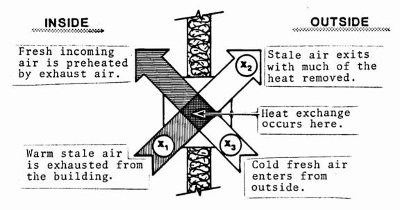
FIG. 2 Schematic Diagram and Flow Stream Nomenclature For An Air-To-Air Heat Exchanger.
