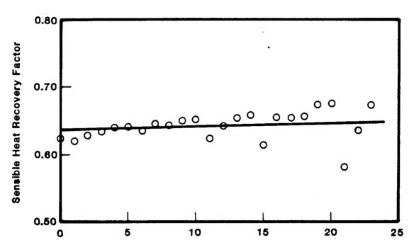
Figure 21: Time Varying Performance of Coil-Loop-Run-Around
