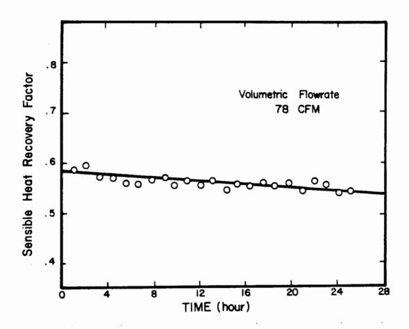
Figure 19: Time Varying Performance of Humid Fire No. 11 Air - to - Air Heat Exchanger
