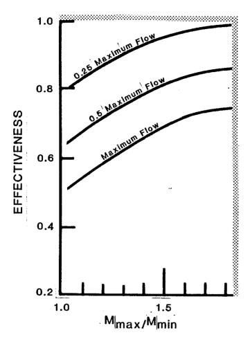
FIG. 4 Variation in Heat Exchanger Effectiveness as a Function of Flow Rate Ratio
