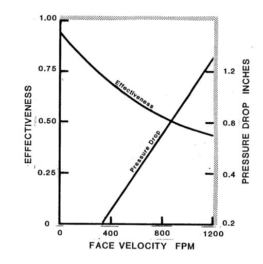
FIG. 5 Variation in Heat Exchanger Effectiveness and Pressure Drop as a Function of Face Velocity
