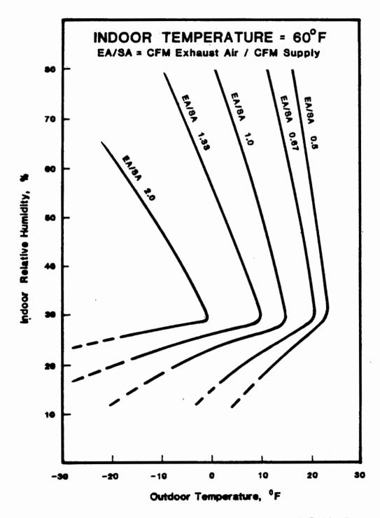
FIG. 7 Frost Threshold Curves For Q-Dot [6] Air-To-Air Heat Exchanger. Operating conditions to the right of the curve should result in no frosting on exhaust side of unit.
