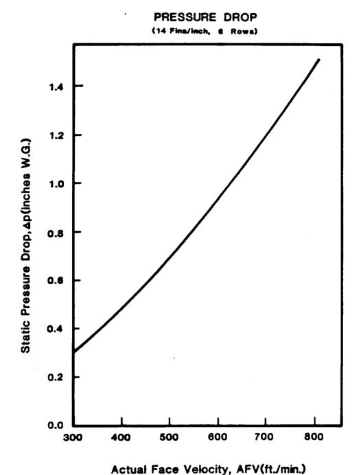
FIG. 24 Static Pressure Drop as a Function of Average Face Velocity for a TRU-120M-6B Q-DOT [6] Heat Tube Heat Recovery Device.
