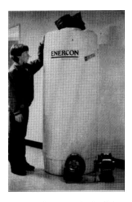
FIG. 13 A Canadian manufactured residential heat exchanger, Enercon, [8], similar in design to the Besant unit. The supply and exhaust fans included with the unit are also shown.
