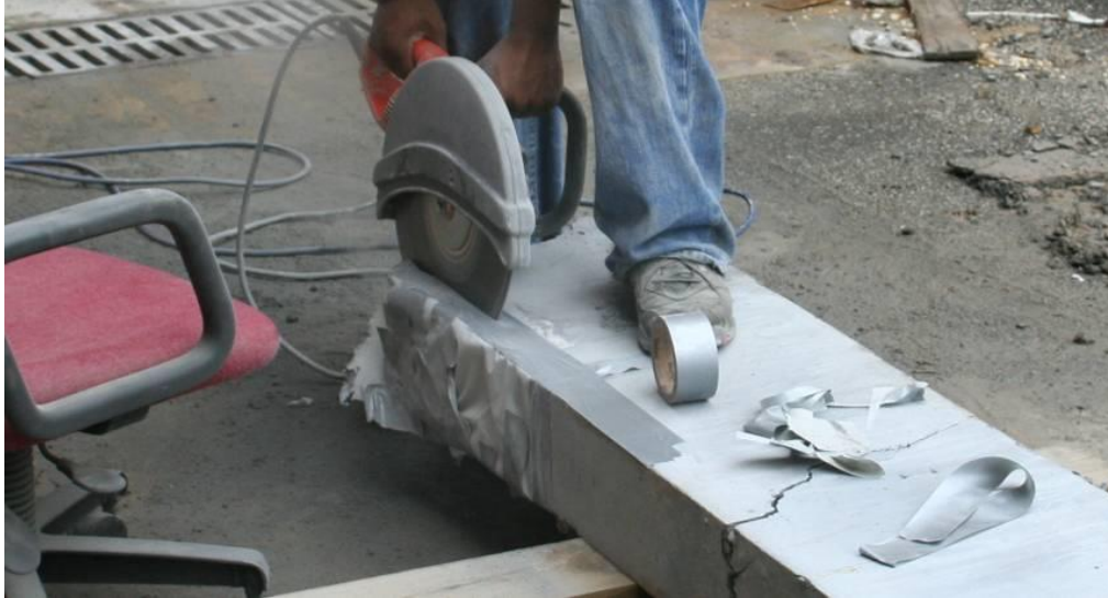
Figure 1. Photo. Extraction of a prismatic specimen from a beam tensile face.
