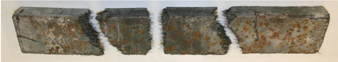
Figure 3. Photo. Failed UHPC tensile prism after the completion of three tension tests.
