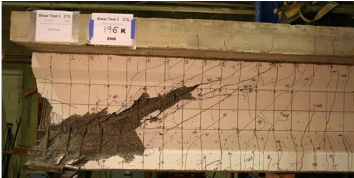
Figure 27. Photo. Shear failure of girder test C7L showing concrete crushing near support.
