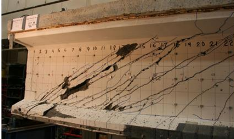
Figure 28. Photo. Shear failure of girder test C8L showing concrete crushing along web.
