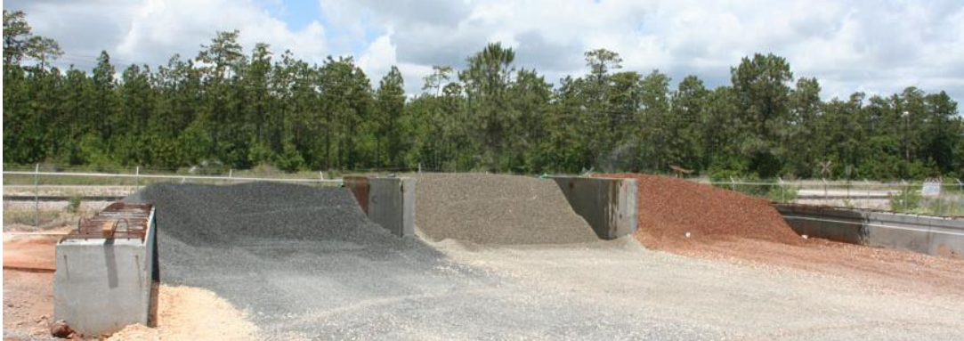
Figure 7. Photo. Lightweight aggregate stockpiles at precaster's facility with continuous sprinklers.
