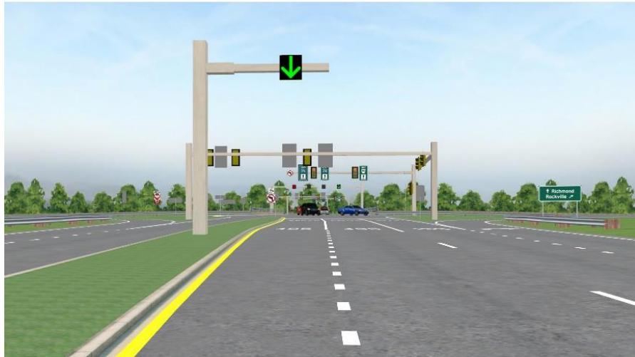
A. Green-arrow CMS over the left-turn bay, indicating it is open to traffic.
