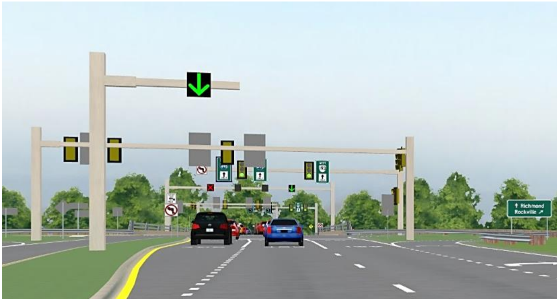
Figure 10. Illustration. Green-arrow CMS above the left-turn bay.
