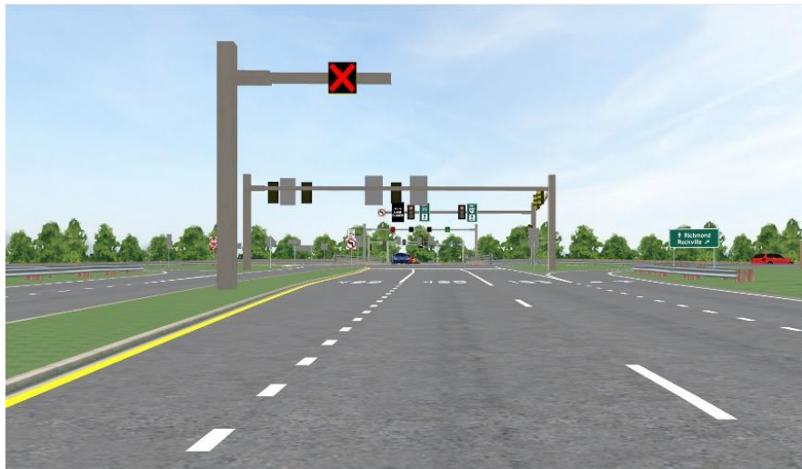
B. Red-X CMS over the left-turn bay, indicating it is closed to traffic.
