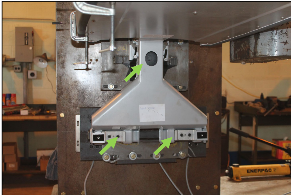
Figure 12 – Table B Pre-Test Photo Depicting Locations of Load Cells
