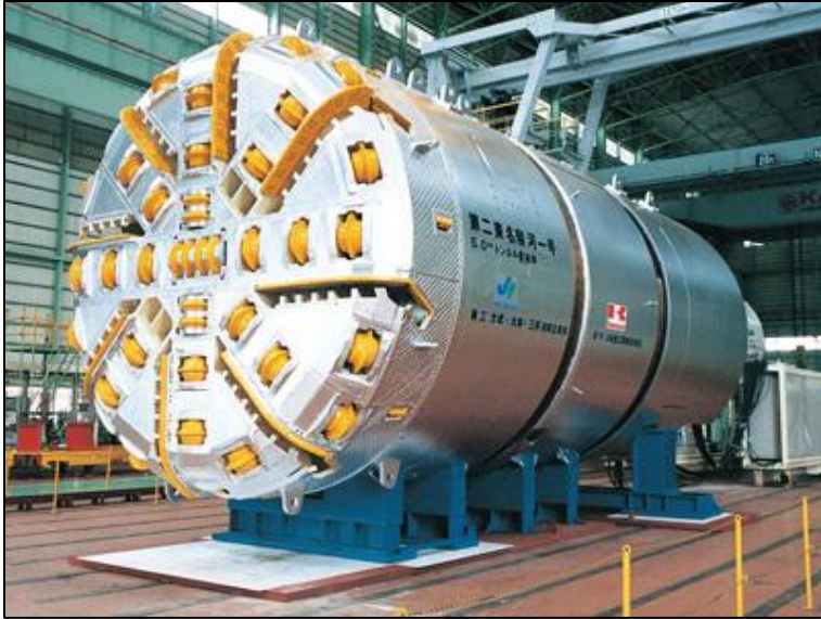
Figure 5 Tunnel Boring Machine: (a) General view of TBM face, (b) TBM disc cutters
